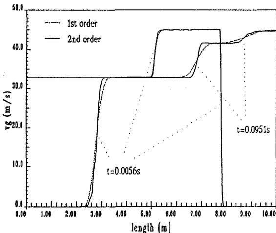
Figure 5: Two-phase shock tube gas velocity.
