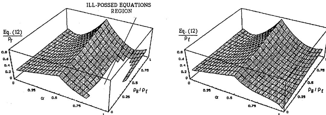
Figure 1: Expression (12) divided by  $\rho_f$  with virtual mass coefficient (13) plotted as a function of  $\alpha$  and  $\rho_g/\rho_f$ . Figure 2: Expression (12) divided by  $\rho_f$  with virtual mass coefficient (14) plotted as a function of  $\alpha$  and  $\rho_g/\rho_f$ .
