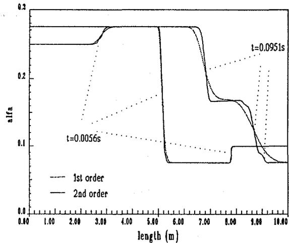
Figure 4: Two-phase shock tube void fraction.
