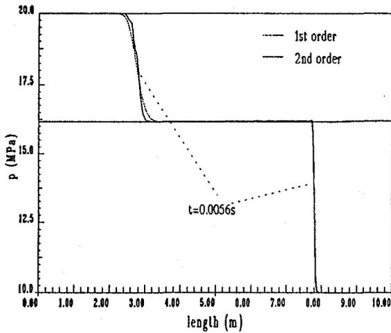
Figure 3: Two-phase shock tube pressure - 1st vs. 2nd order scheme.
