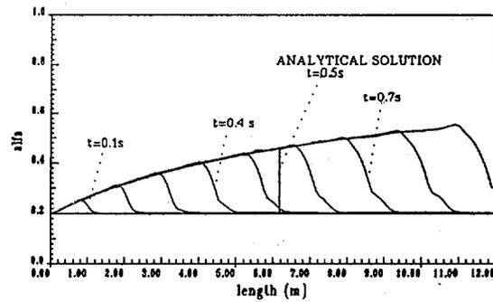
Figure 7: Water Faucet problem. Development of the void fraction profile.
