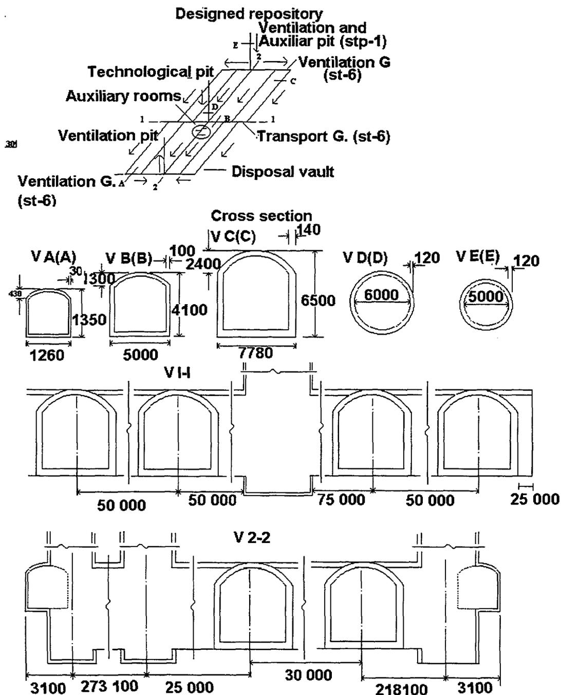
FIG. 1. Layout of designed repository.
