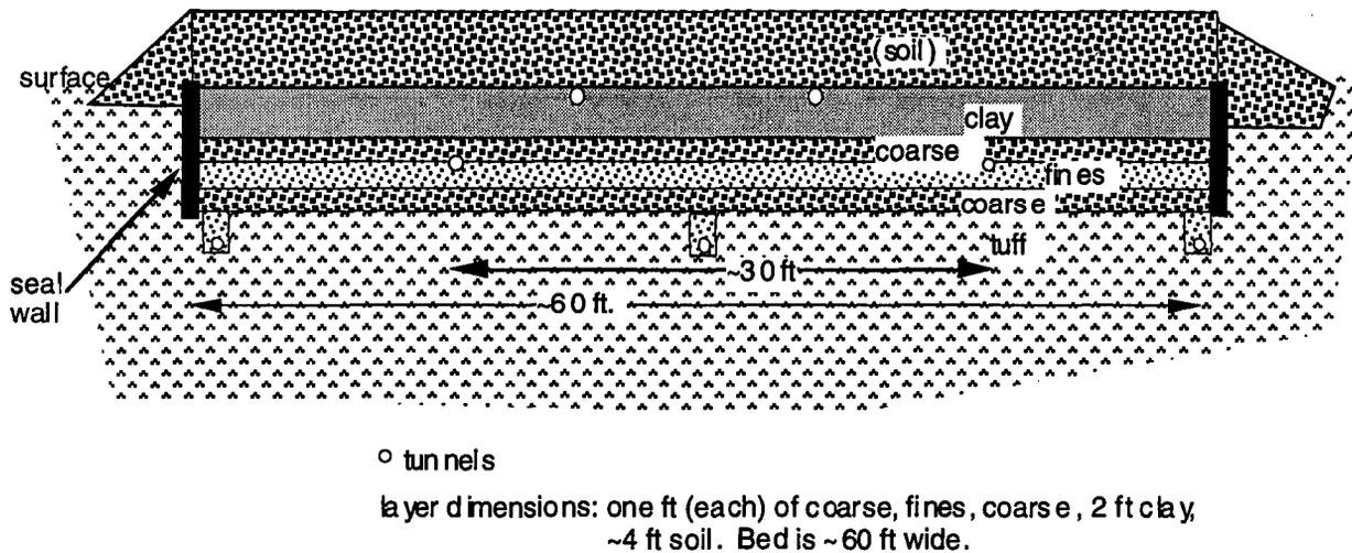
Figure 2. Dimensions of the prototype test bed
