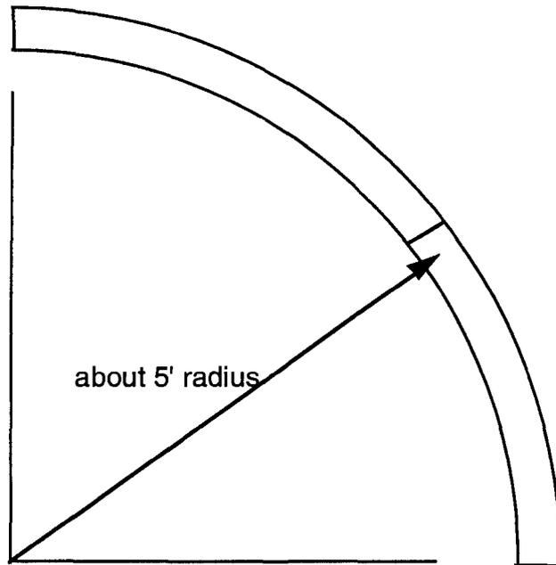
Convenient handling requires a pipe section about 4 ft. long which would lead to about a 45 degree turn of each section. The pipe i.d. should be about the same as standard pipe. Section connections can be of other materials supplied later.
