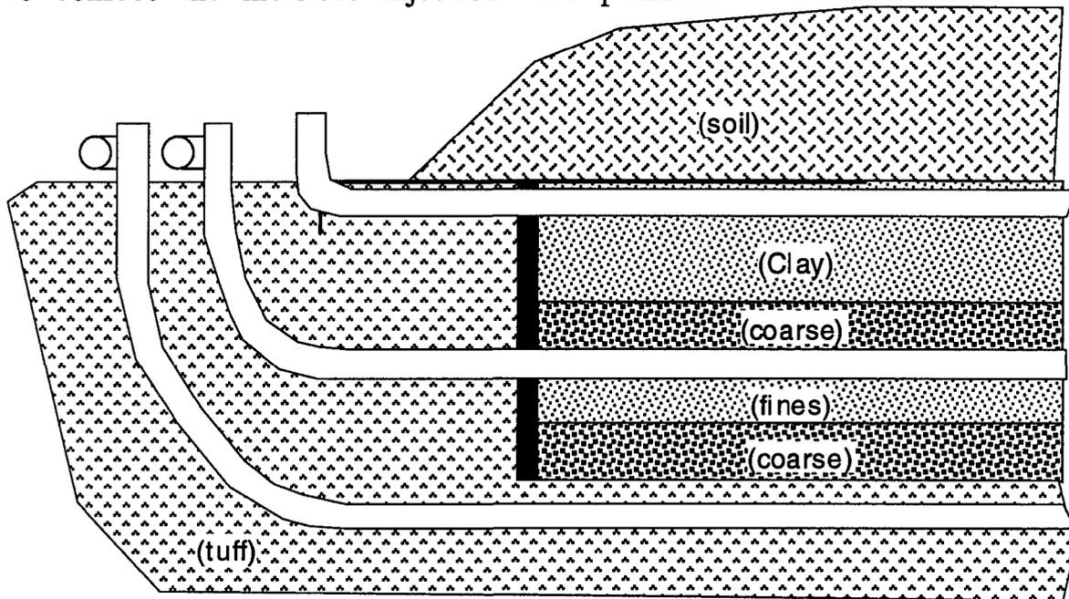
Figure 3. Access pipes to tunnels in testbed
