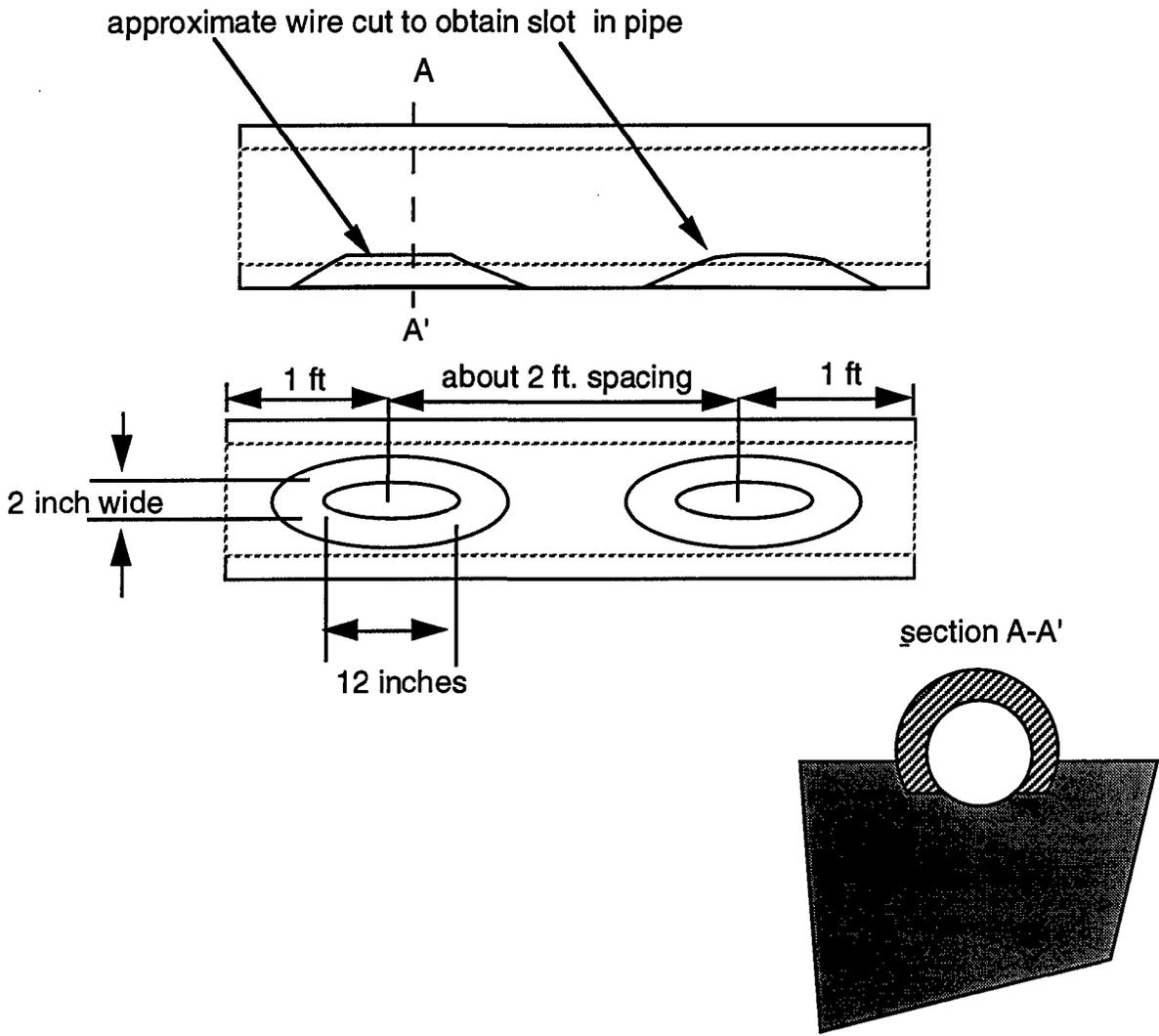
Figure 2. The slotted pipe tunnel
