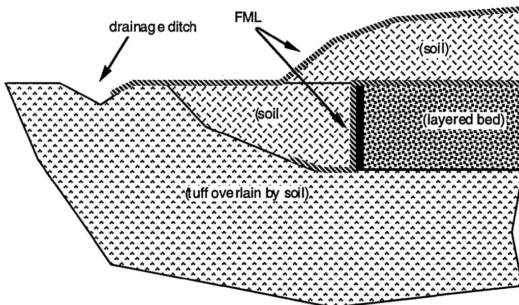
Figure 4. Wall and surface seal geometry of layered bed
