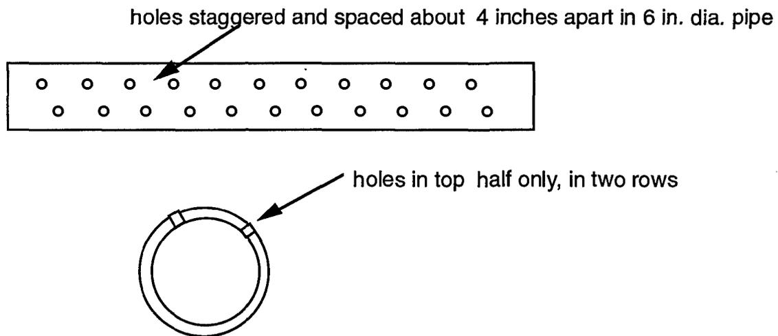
**Figure 4. Perforation geometry. Holes are to be of about 0.25 in. diameter with minimum sharp projection on the inside.**
