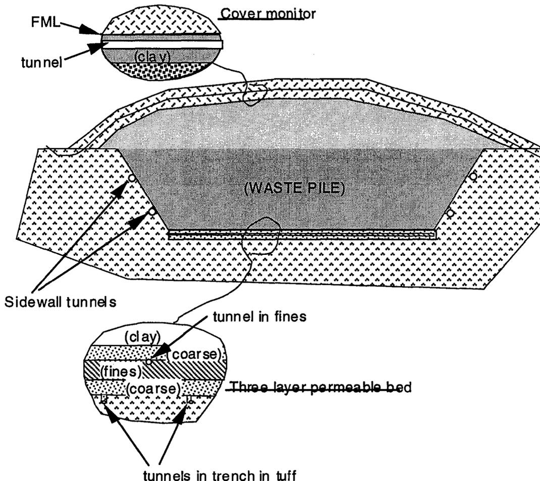
The sidewall monitoring was also not explicitly included in the prototype test except as the basic function is inherent in the lower tunnels of the permeable bed system. The permeable bed and the cover monitoring were included in the test bed in a manner to allow both to be constructed with the minimum cost yet provide a full reproduction of the hydrologic circumstances.
