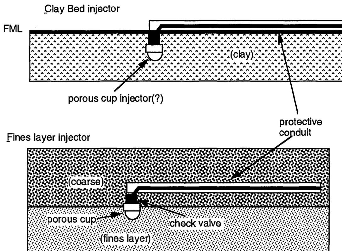
Figure 8c. Injection point geometry (all tubing lines parallel to the tunnels)
