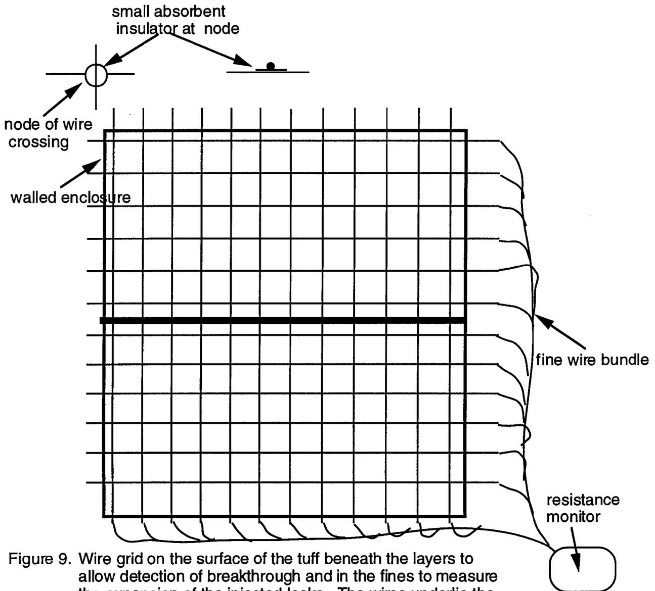
Figure 9. Wire grid on the surface of the tuff beneath the layers to allow detection of breakthrough and in the fines to measure the expansion of the injected leaks. The wires underlie the tunnels in the fines, and overlie the tunnels in the tuff.
