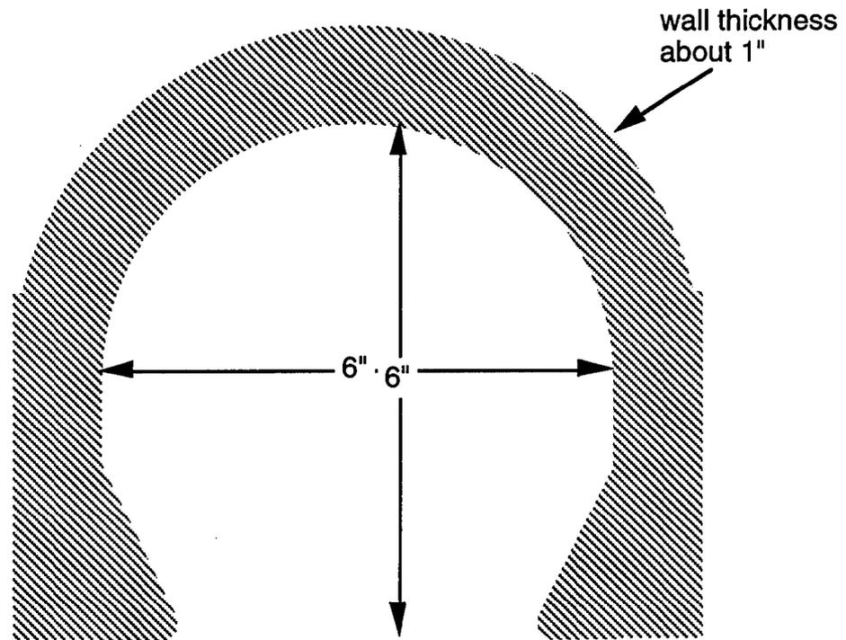
Dimensions approx., Made from standard pipe section as convenient and to allow for testing on the three line loading machine. Normal firing.
