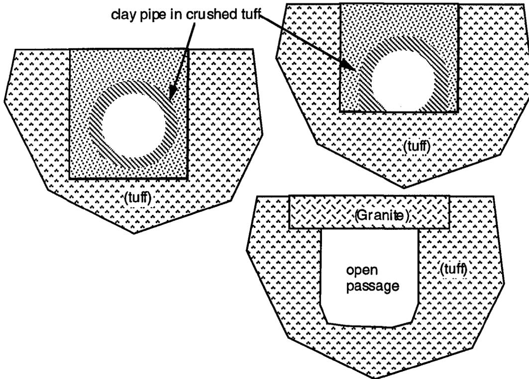
Figure 5. Possible tunnel geometries
