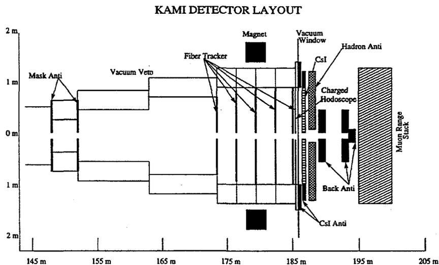
Figure 6: Schematic of the proposed KAMI detector for  $K_L \rightarrow \pi^0 \nu \bar{\nu}$ .
