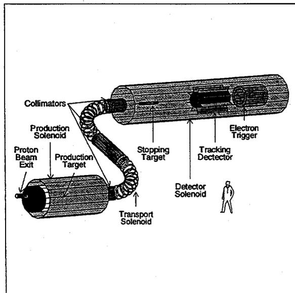
Figure 14: Schematic layout of the MECO detector.
