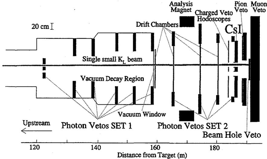
Figure 4: Schematic of the KTeV detector as configured for special  $K_L \rightarrow \pi^0 \nu \bar{\nu}$  run.
