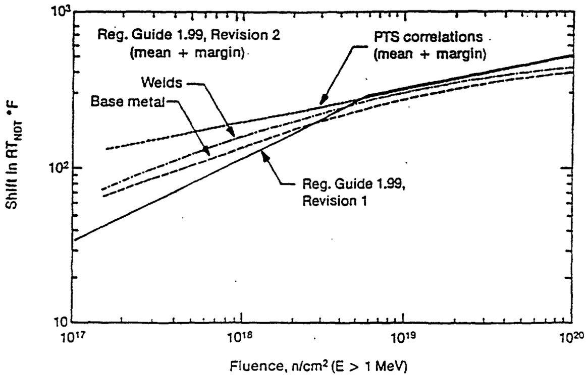
Fig. 3 Comparison of shift predictions for welds and base metal (0.35 wt% Cu and 0.60 wt% Ni) calculated using Revisions 1 and 2 of Regulatory Guide 1.99 and other PTS correlations.
