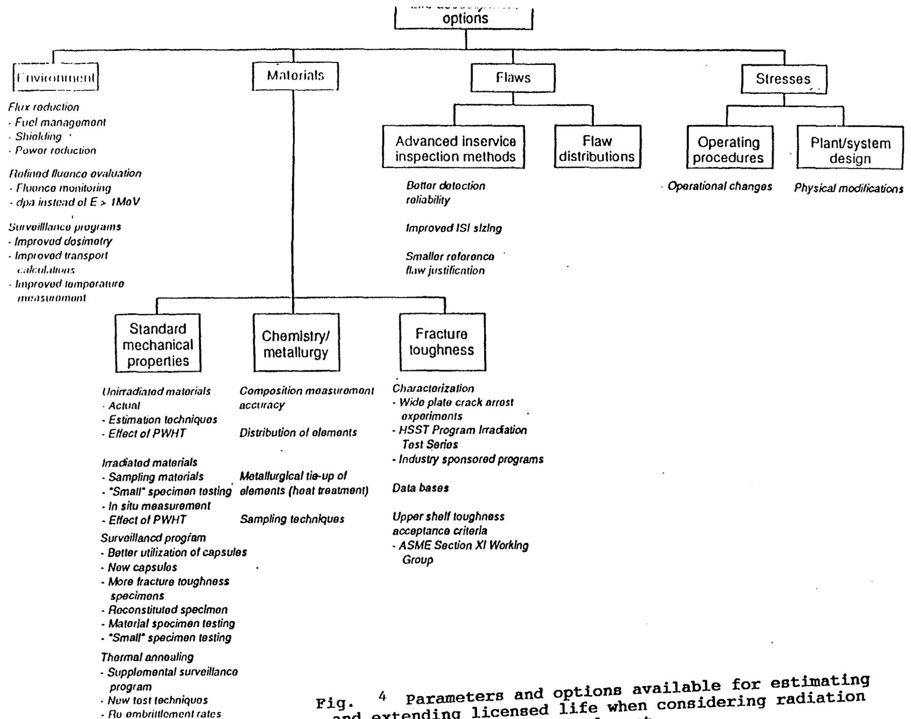
Fig. 4 Parameters and options available for estimating and extending licensed life when considering radiation embrittlement.
