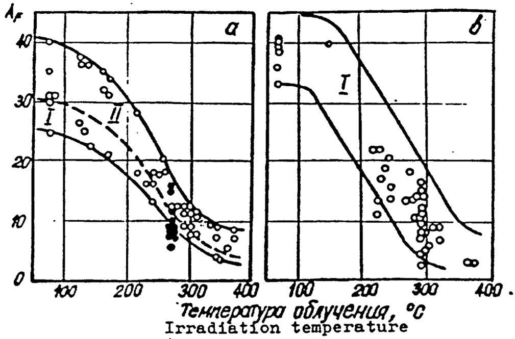
Fig. 6 Effect of irradiation temperature on radiation embrittlement factor of weld metal of steels 15X2MOA (a), and 15X2HMOAA (Cu  $\leq$  0.08%; P  $\leq$  0.012%) (b)
