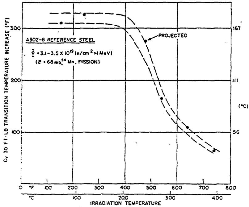
Fig. 2 Effect of irradiation temperature on transition temperature increase for an A302-B reference steel [17].
