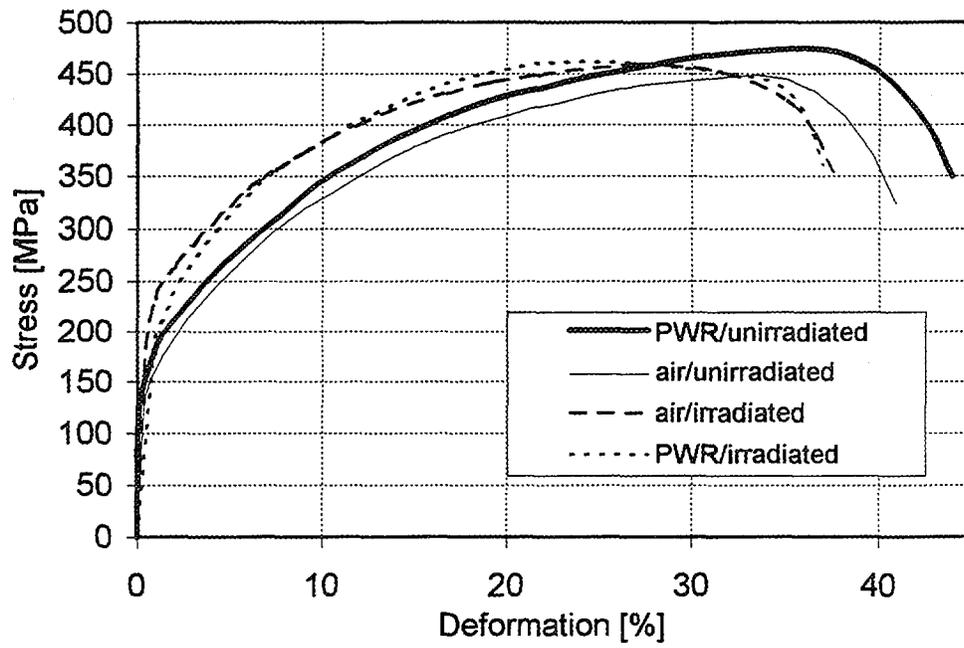
Fig.9: Stress - deformation line of the loading of 08Kh18N10T steel preirradiated to the fluence of  $1 \times 10^{20}$  n/cm<sup>2</sup> and non - irradiated.
