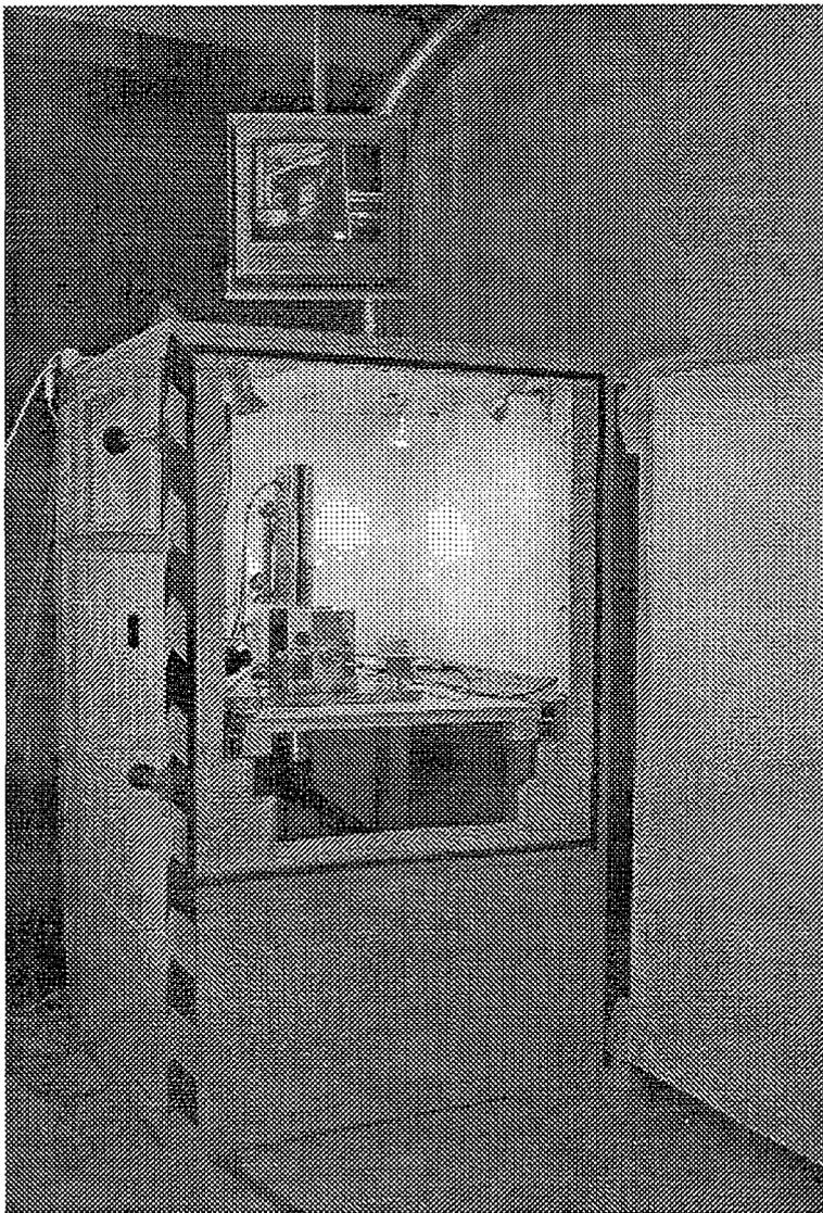
Fig.8: Hot cell with SEM
