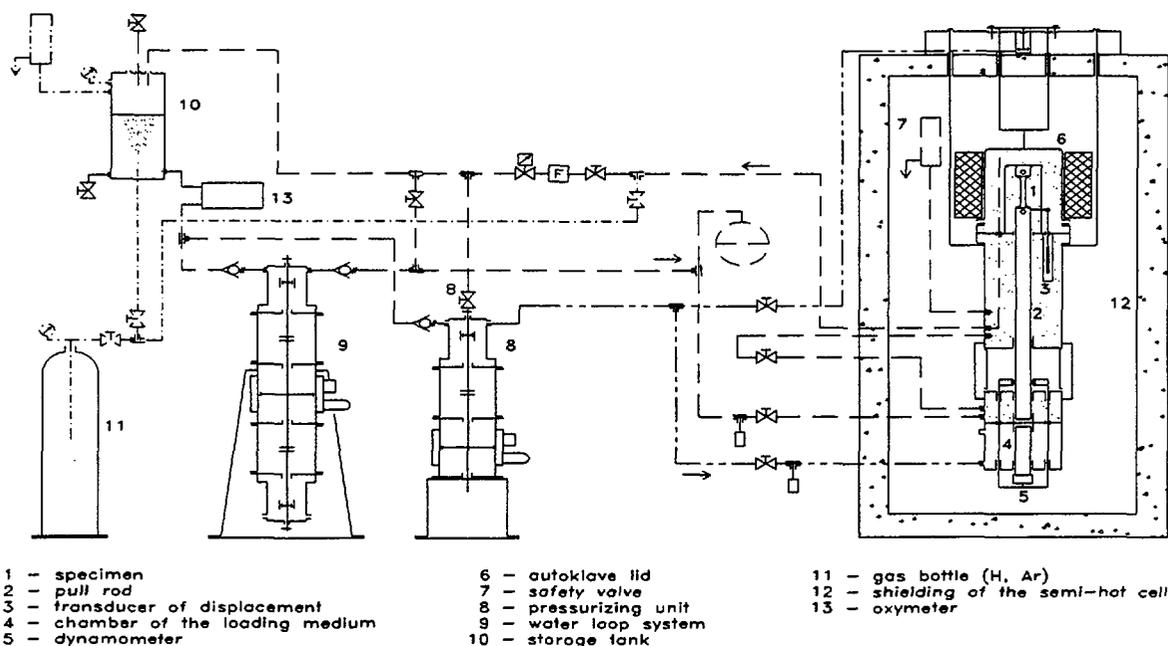
Fig. 4: Hot cell SSRT testing system
