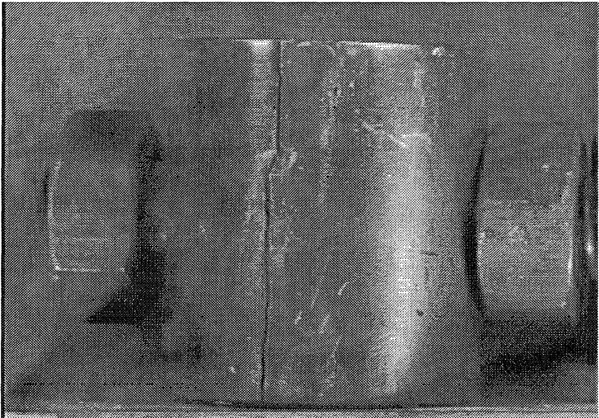
Fig.10: Surface of C - ring tested in pile after preirradiation
