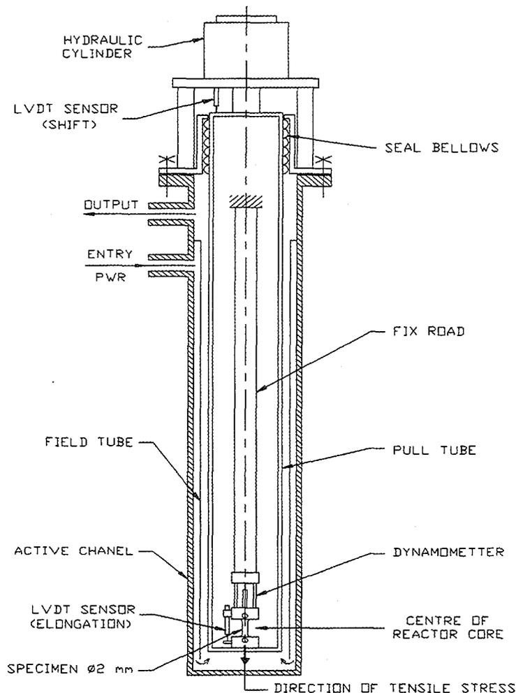
Fig. 5: Scheme of in-pile loading facility
