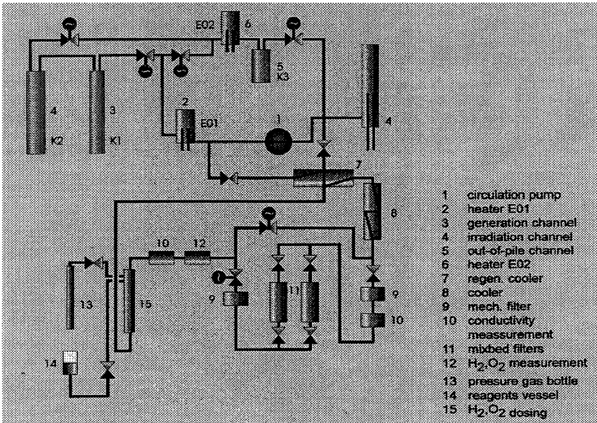
Fig.2: Boiling water loop
