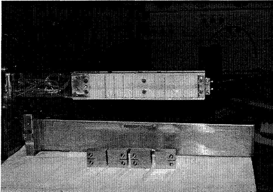
Fig.3: Irradiation rig for four CT specimens
