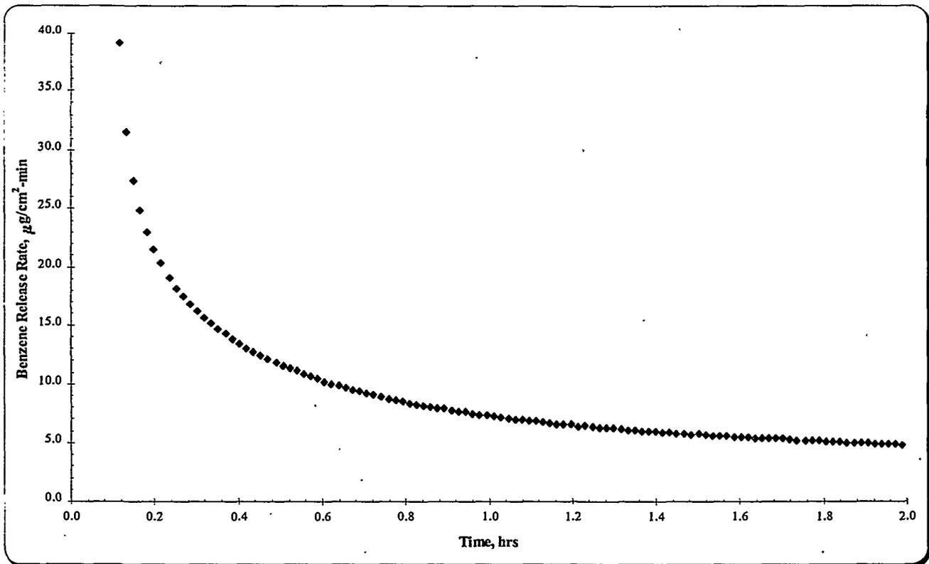
Figure 10a. Benzene Release from Quiescent Slurry Homogenized with 17,068-ppm Benzene
