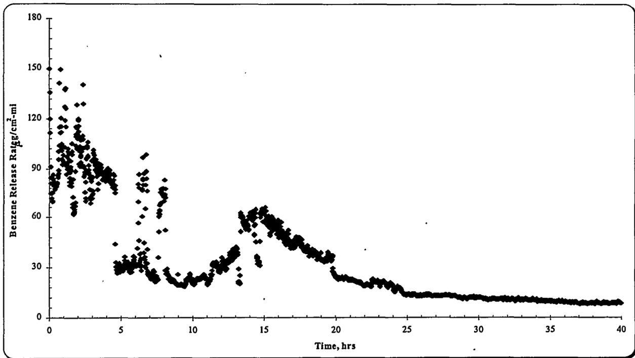
Figure 16b. Benzene Release (45°C) from Agitated Slurry Homogenized with 20,653-ppm Benzene
