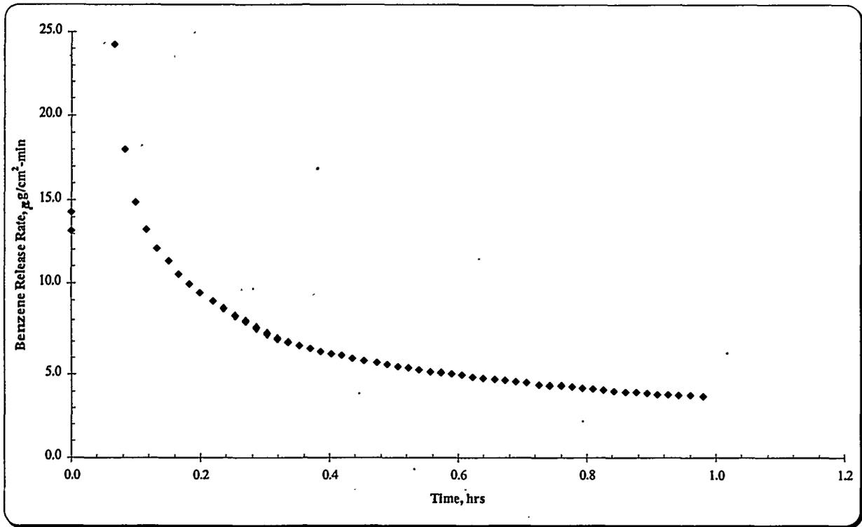
**Figure 12a.** Benzene Release from Quiescent Slurry Homogenized with 5,408-ppm Benzene
