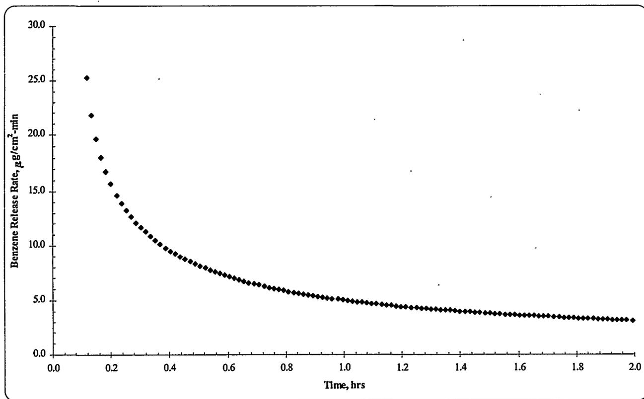
**Figure 11a.** Benzene Release from Quiescent Slurry Homogenized with 8,535-ppm Benzene
