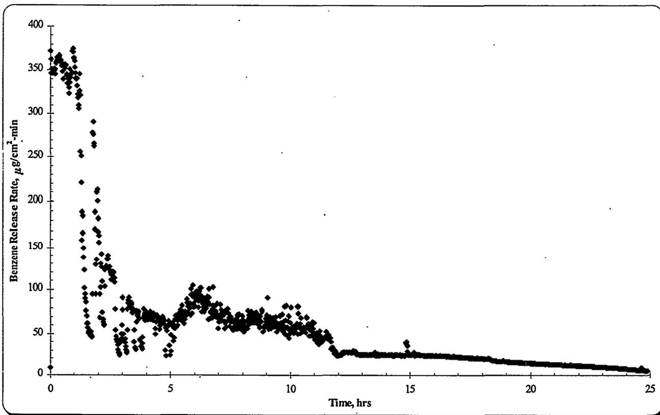
**Figure 15b.** Benzene Release (45°C) from Agitated Slurry Homogenized with 19,024-ppm Benzene
