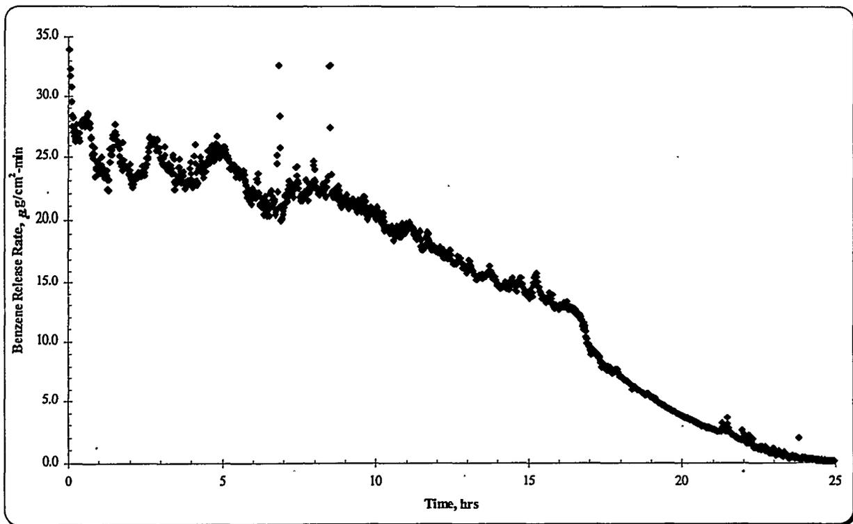
**Figure 12b.** Benzene Release from Agitated Slurry Homogenized with 5,408-ppm Benzene
