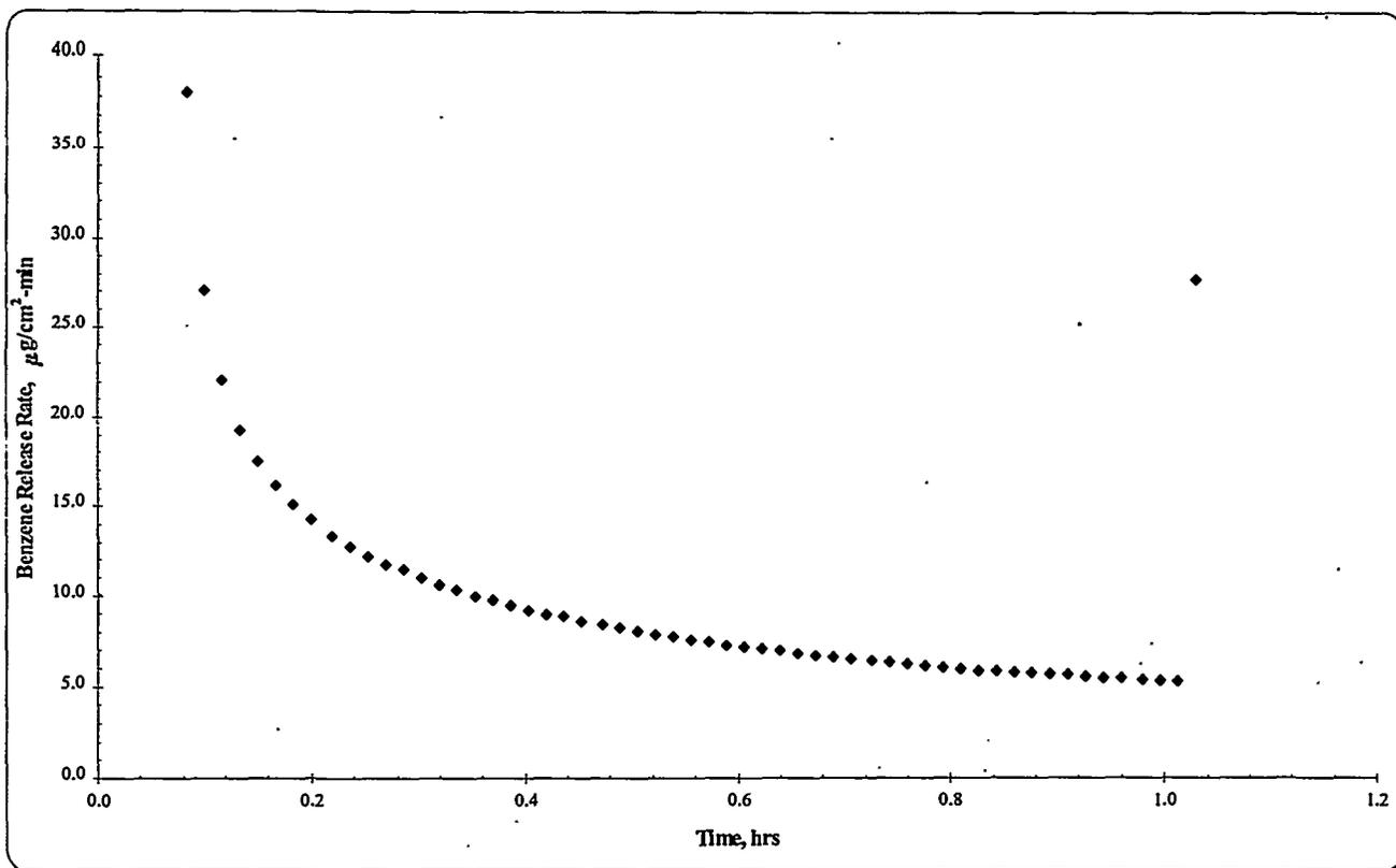
Figure 9a. Benzene Release from Quiescent Slurry Homogenized with 16,624-ppm Benzene
