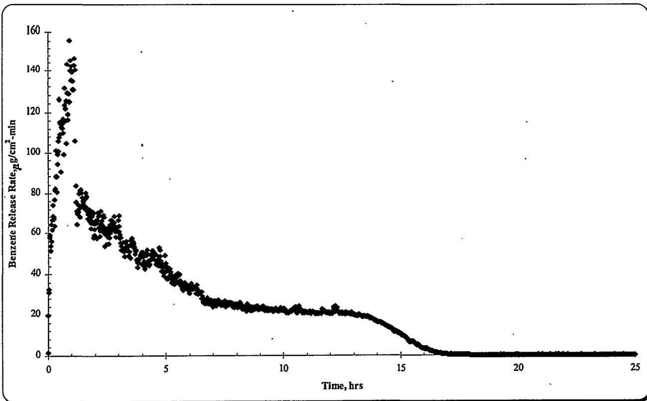
Figure 8b. Benzene Release from Agitated Slurry Containing 8,109-ppm Freshly Added Benzene
