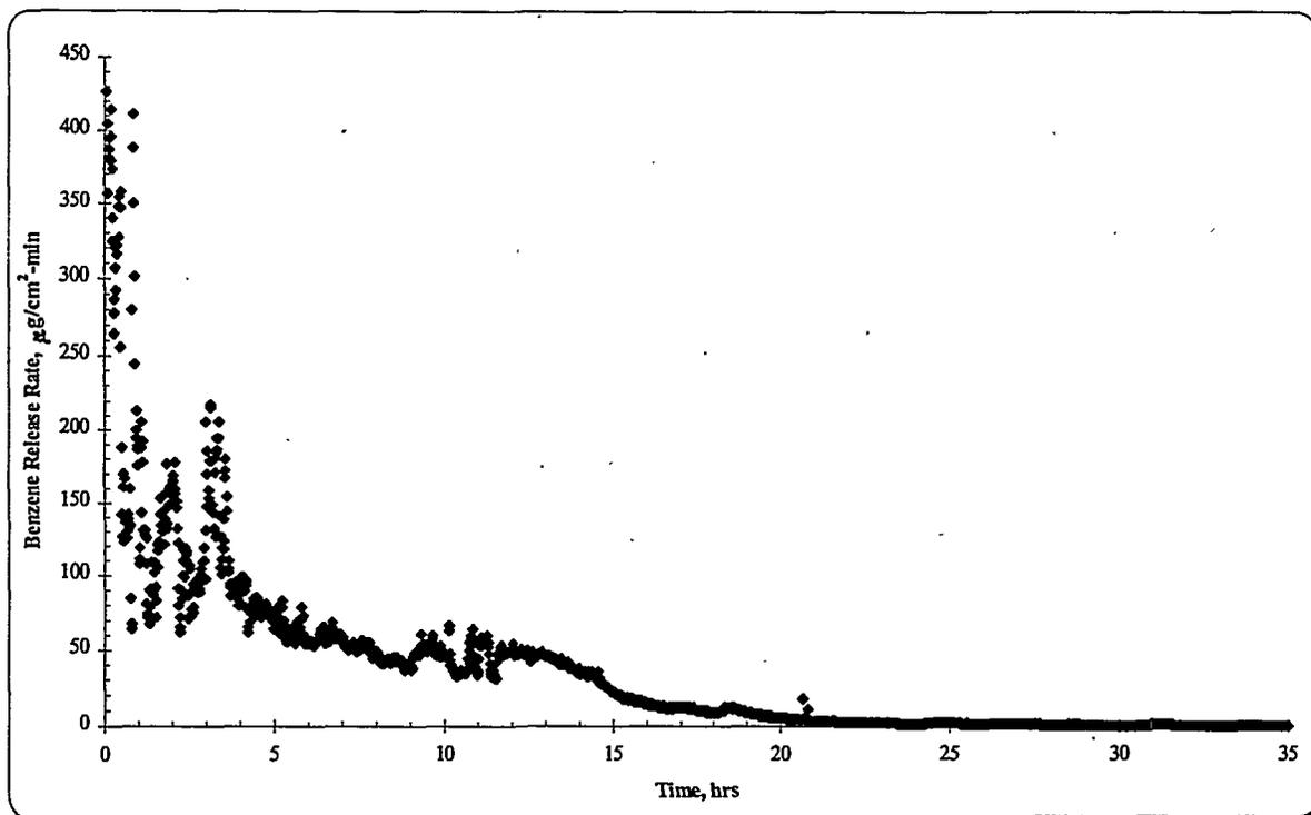
**Figure 14b.** Benzene Release (45°C) from Agitated Slurry Containing 17,323-ppm Freshly Added Benzene
