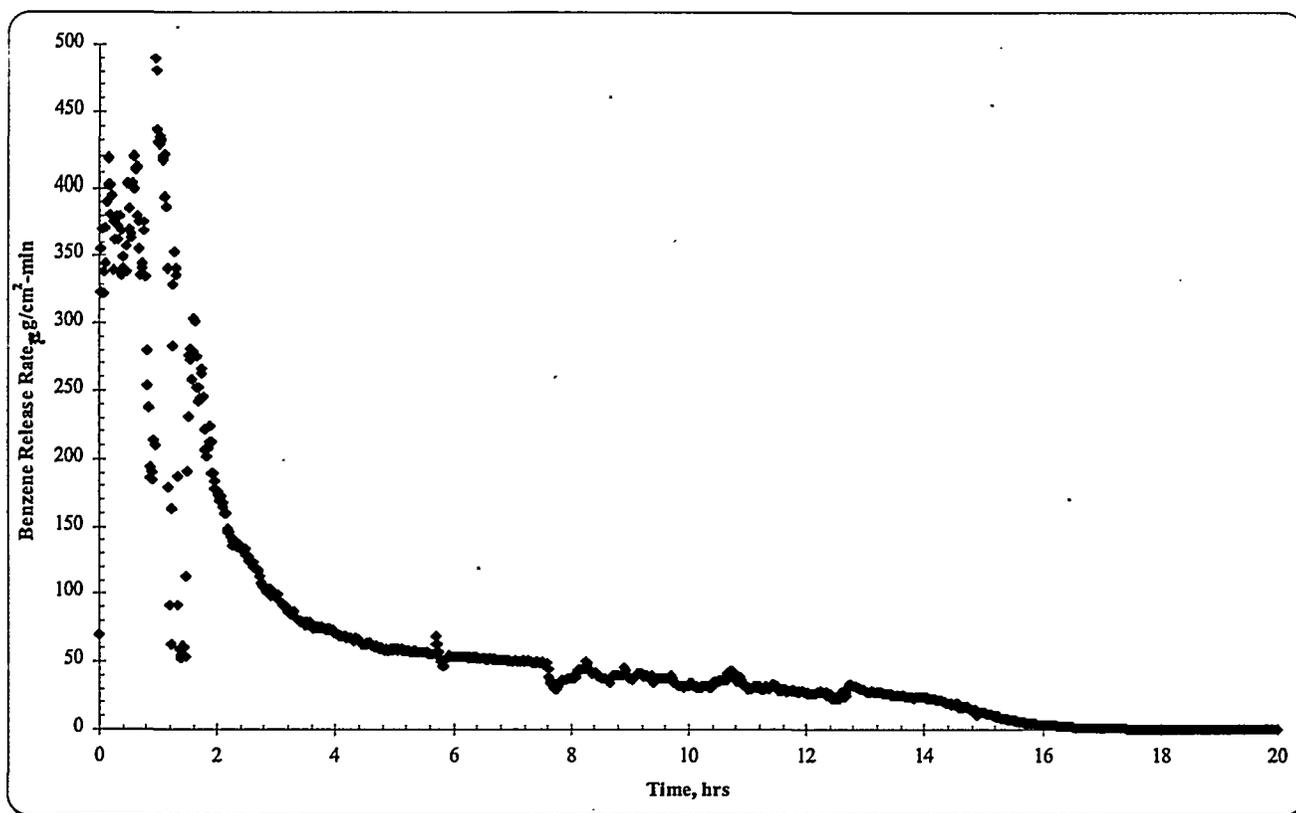
**Figure 5b.** Benzene Release from Agitated Slurry Containing 15,730-ppm Freshly Added Benzene
