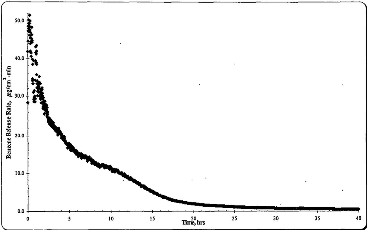
Figure 18b. Benzene Release from Agitated DEMO Column Slurry Containing Benzene Generated *In Situ*
