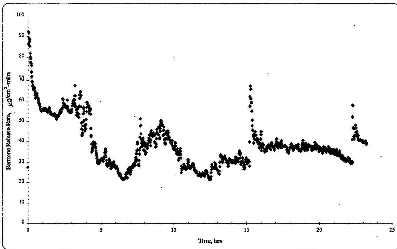
**Figure 9b.** Benzene Release from Agitated Slurry Homogenized with 16,624-ppm Benzene
