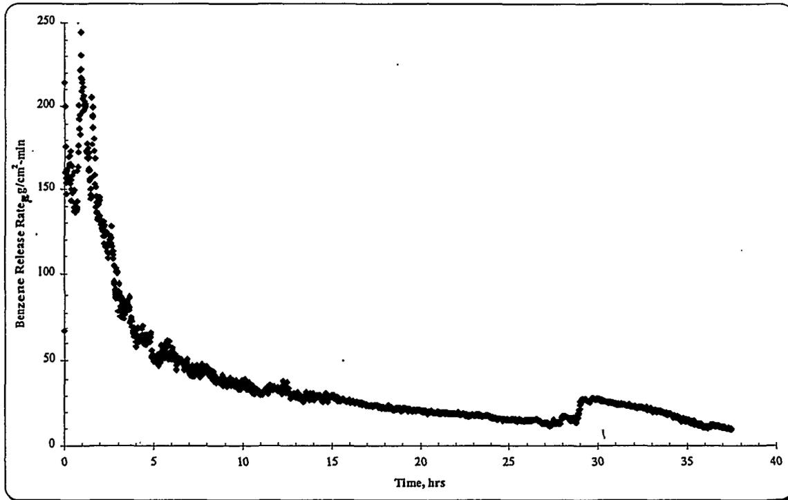
**Figure 17b.** Benzene Release (35°C) from Agitated Slurry Homogenized with 18,522-ppm Benzene
