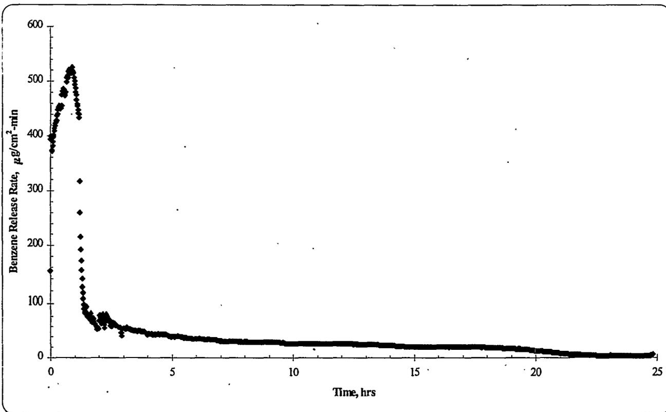
**Figure 7b.** Benzene Release from Agitated Slurry Containing 16,585-ppm Freshly Added Benzene
