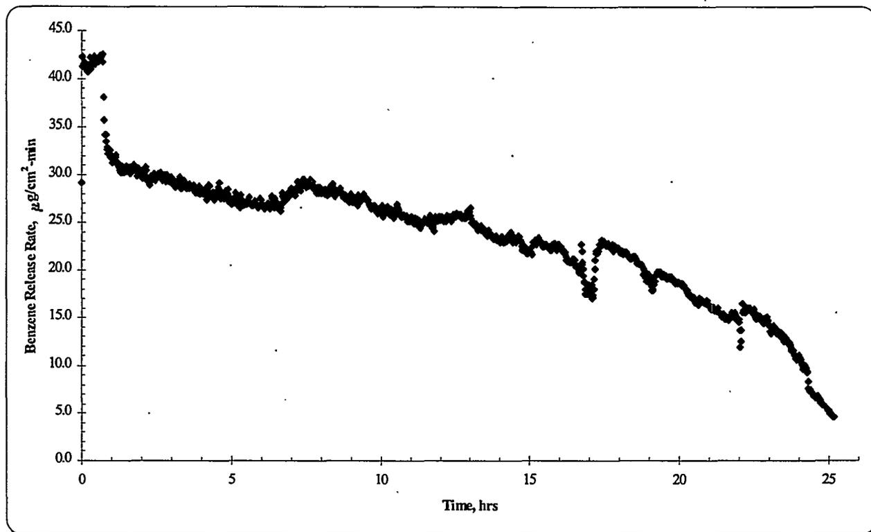
**Figure 11b.** Benzene Release from Agitated Slurry Homogenized with 8,535-ppm Benzene
