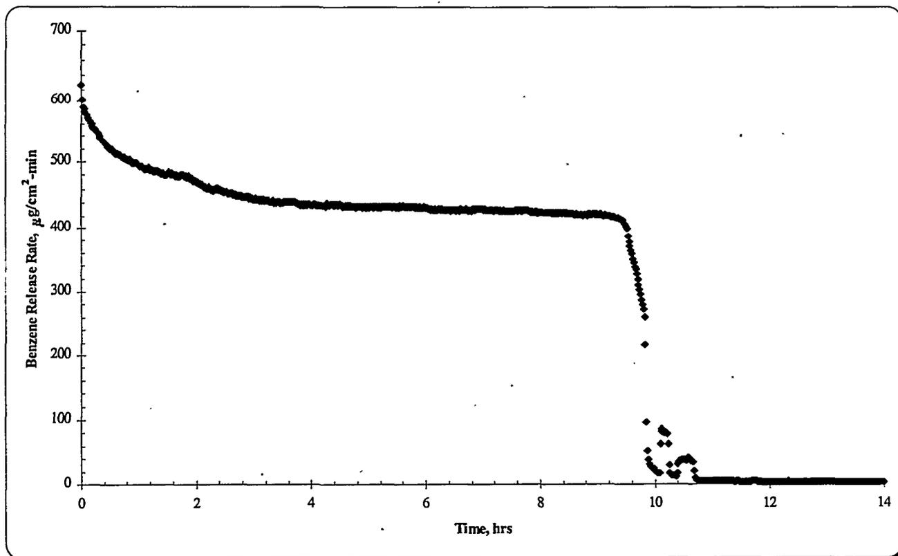
Figure 4. Benzene Release from Pure Benzene Layer on KTPB Slurry
