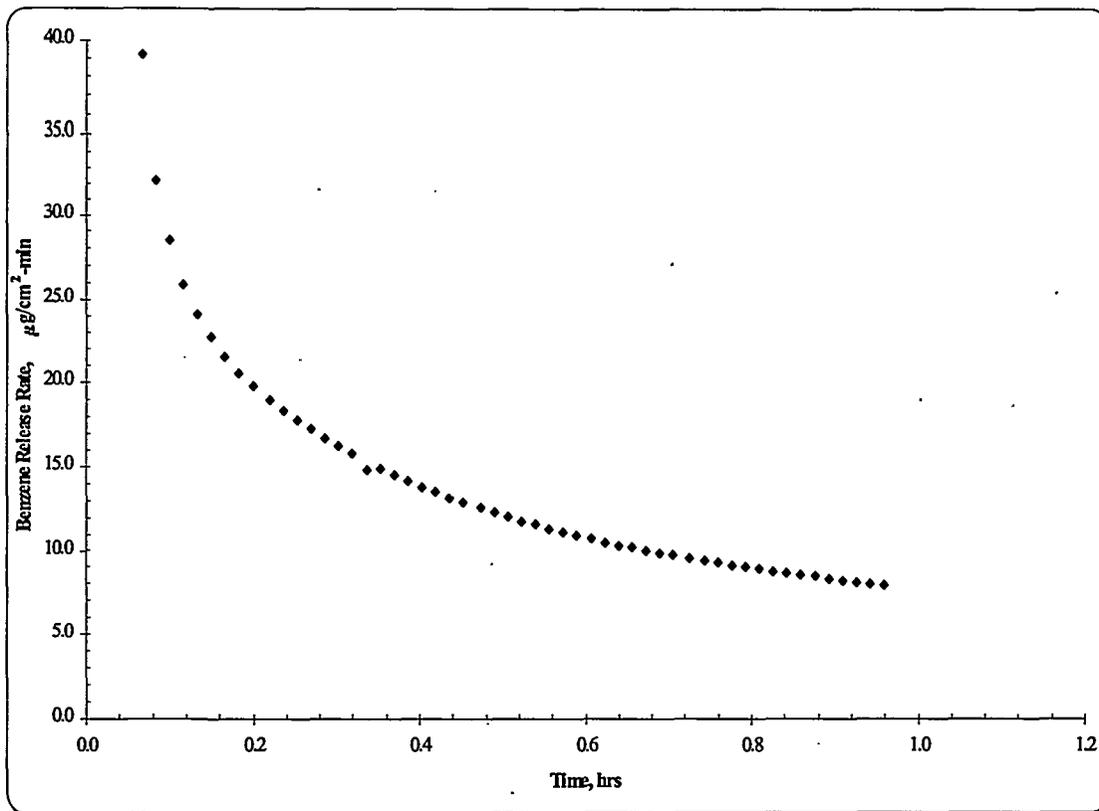
Figure 17a. Benzene Release (35°C) from Quiescent Slurry Homogenized with 18,522-ppm Benzene
