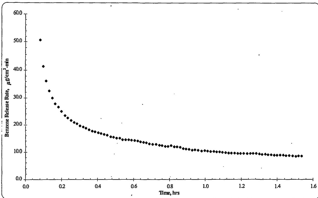
Figure 13a. Benzene Release from Quiescent Slurry Homogenized with 9,598-ppm Benzene and Containing 8,951-ppm Freshly Added Benzene
