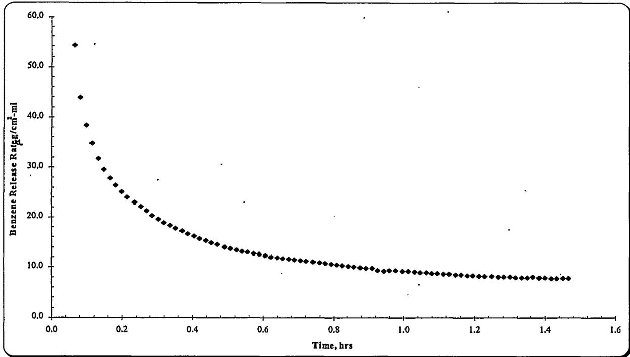
Figure 16a. Benzene Release (45°C) from Quiescent Slurry Homogenized with 20,653-ppm Benzene
