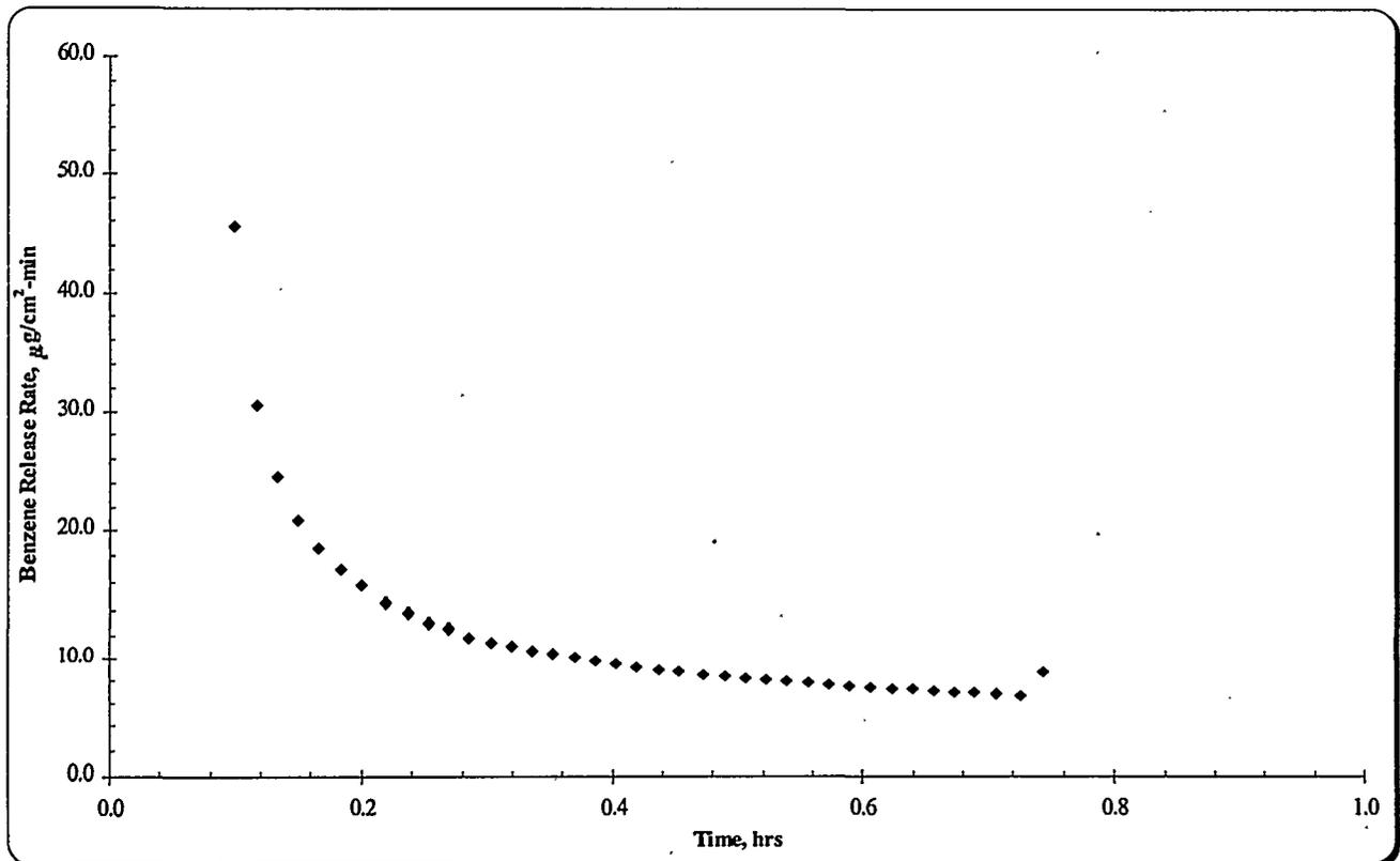
Figure 15a. Benzene Release (45°C) from Quiescent Slurry Homogenized with 19,024-ppm Benzene
