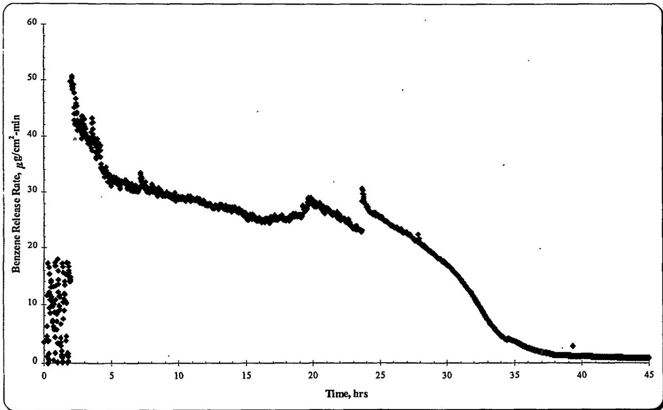
Figure 10b. Benzene Release from Agitated Slurry Homogenized with 17,068-ppm Benzene
