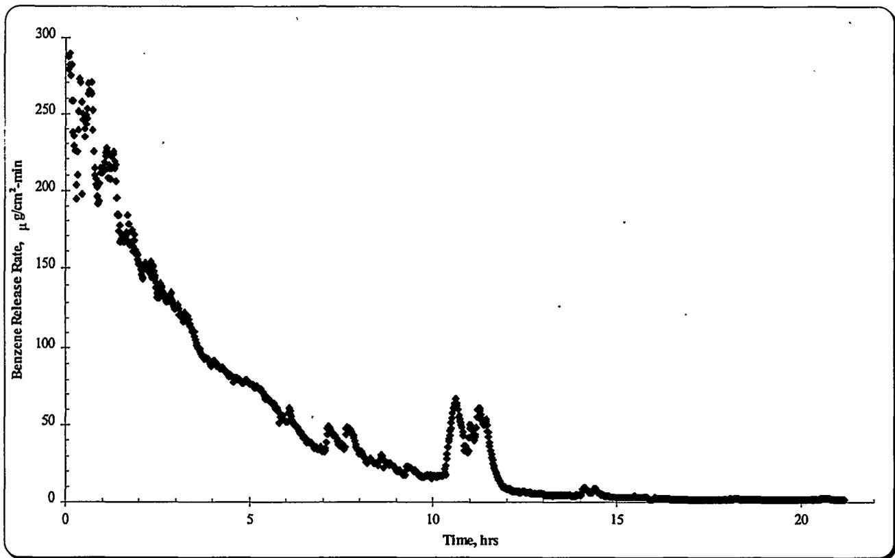
**Figure 13b.** Benzene Release from Agitated Slurry Homogenized with 9,598-ppm Benzene and Containing 8,951-ppm Freshly Added Benzene
