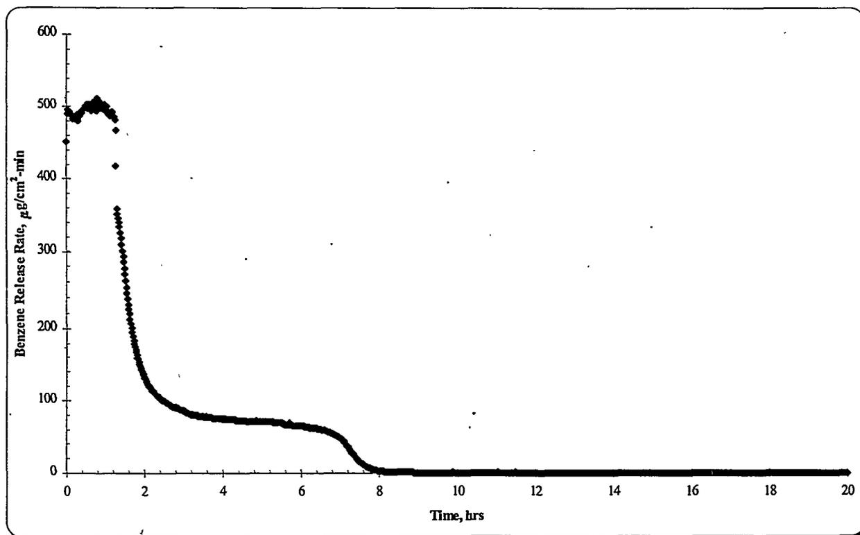
Figure 6b. Benzene Release from Agitated Slurry Containing 16,105-ppm Freshly Added Benzene
