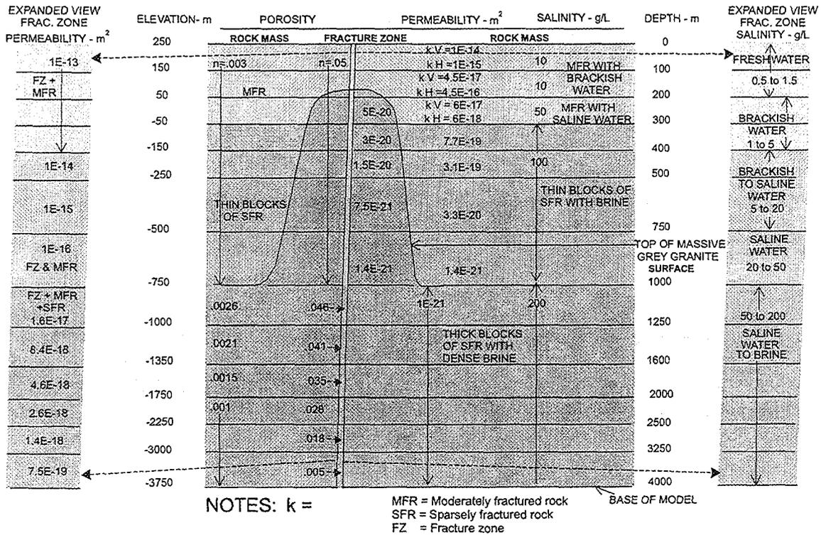
FIGURE 6: A Schematic Section of the Permeability, Porosity and Salinity Distributions in the Fracture Zones, Moderately and Sparsely Fractured Rock with Depth at WRA
