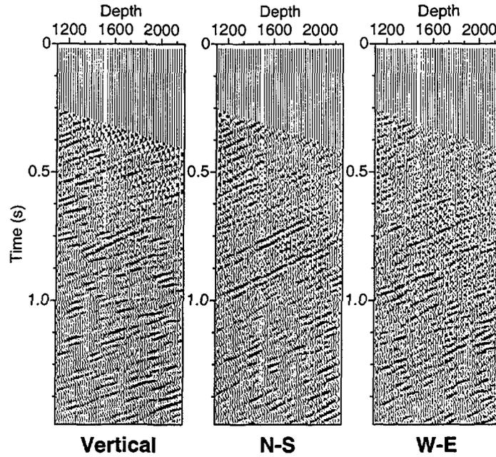
*Figure 4-1 Three component data from the SG-4 borehole showing a clear dipping P- to S- wave converted reflection. The source was offset from the wellhead by 31 m to the east and 839 m to the north.*
