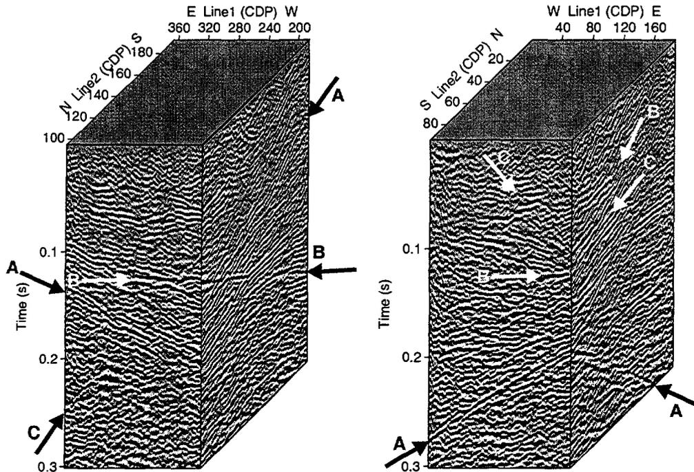
Figure 5-2 N-S and W-E seismic profiles merged where they cross and viewed from the NW (left) and SE (right).
