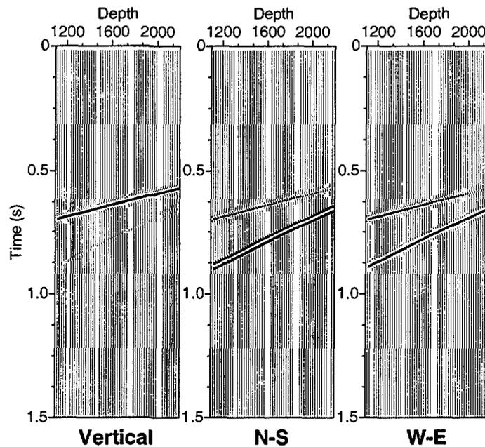
*Figure 4-2 Synthetic data from simple modelling of the P- to S- wave converted event in Figure 4-1. The model consists of an interface dipping  $30^\circ$  to the east, striking N-S, and intersecting the borehole at 2900 m. The elastic parameters were  $V_p=6100$  m/s,  $V_s=3500$  m/s,  $\rho=2700$  kg/m<sup>3</sup> for layer 1 and  $V_p=5500$  m/s,  $V_s=2500$  m/s,  $\rho=2500$  kg/m<sup>3</sup> for layer 2.*
