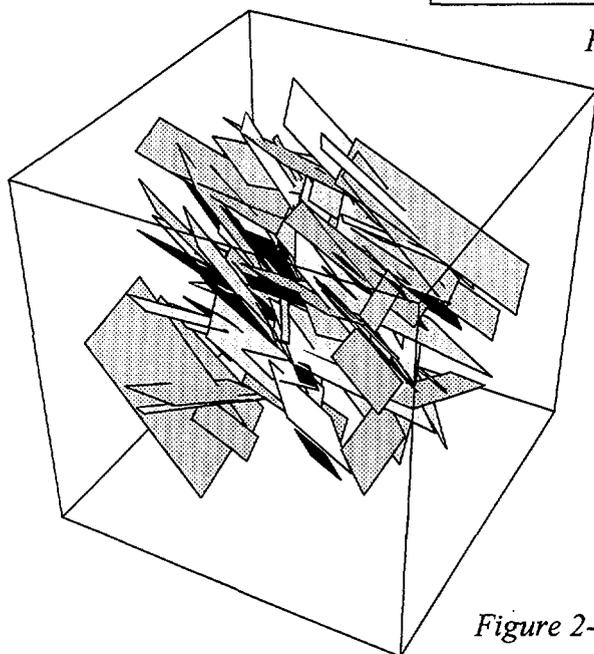
Figure 2-4 Example of a single-family stochastic fracture network.
