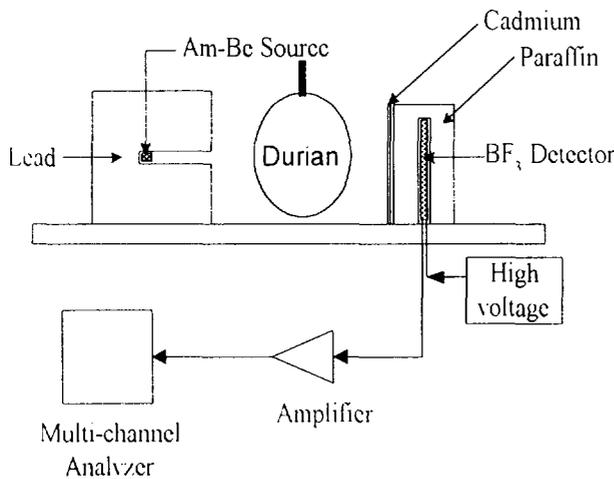
Figure 3 The arrangement of Neutron Transmission technique.
