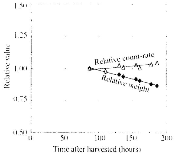
Figure 6 The relation between relative weight with time after harvested and relative count rate from the Neutron Transmission technique.
