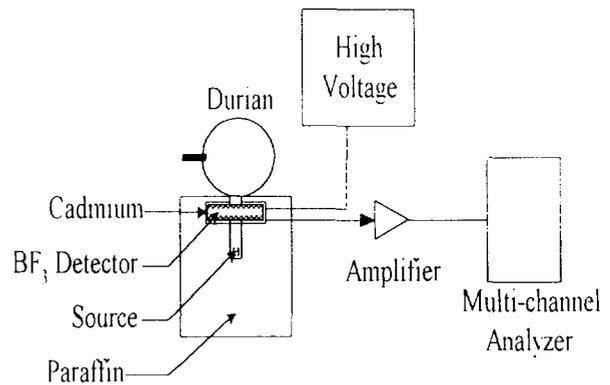
Figure 4 The arrangement of Neutron Reflection technique.
