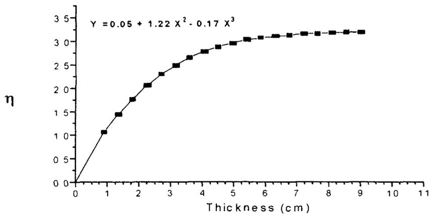
Fig. 4 Excess count rate dependence of the material thickness.
