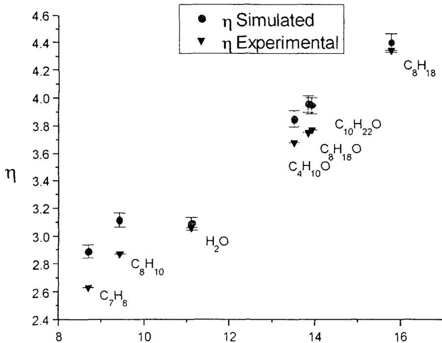
Fig.5 Behaviour of the excess count rate vs. H (w%) for some pure hydrocarbons and alcohols
