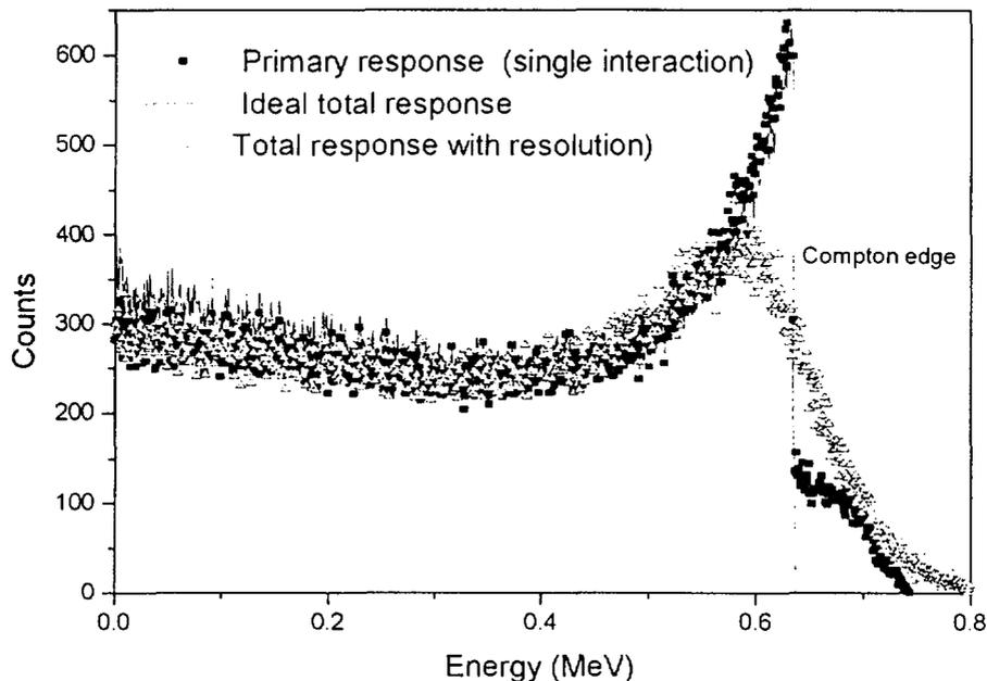
Fig. 3 NE-213 detector simulated response function for gamma radiation.
