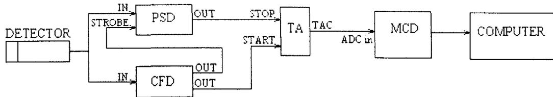
Fig. 2. Electronic scheme for time resolution measurement.
