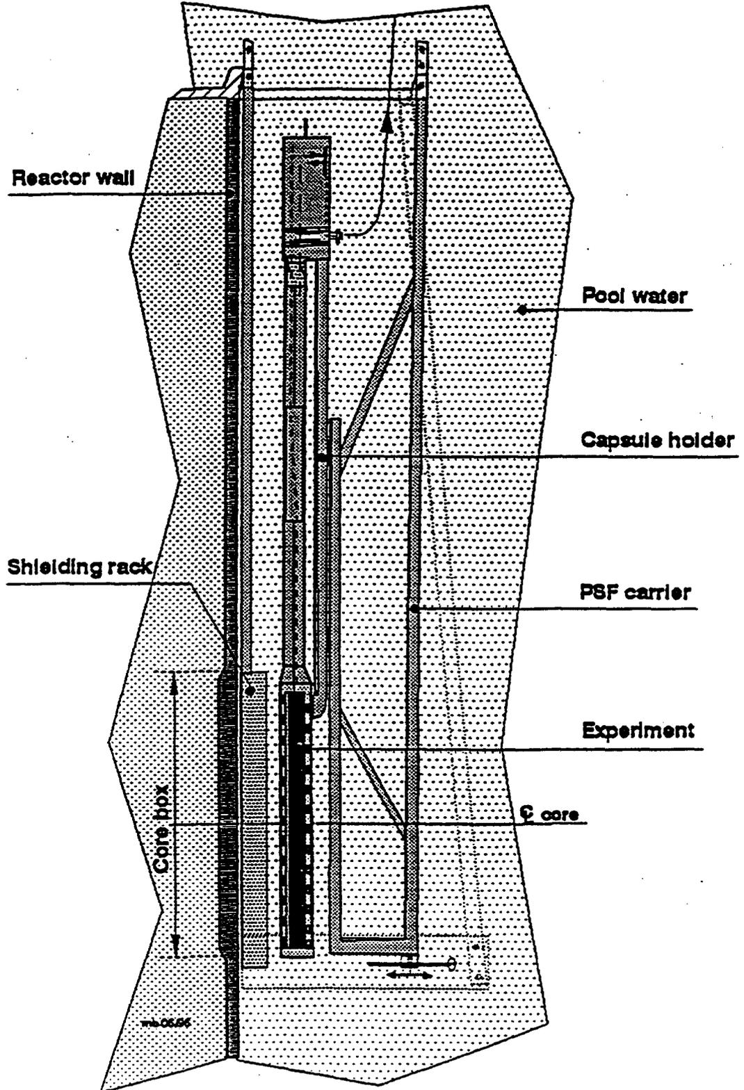
Figure 2. View of the LYRA facility in the PSF of the HFR
