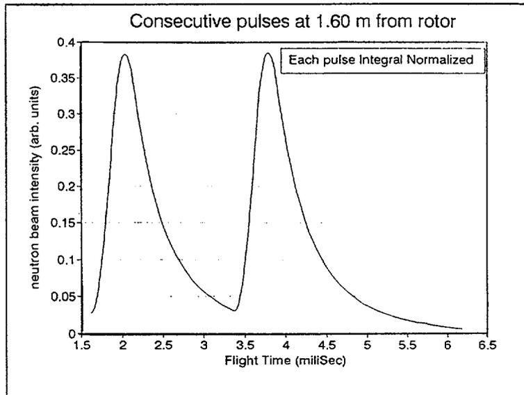
FIG. 5. Consecutive pulses at 1.60 m from rotor.
