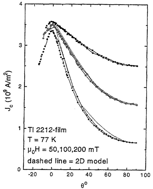
Fig. 4.  $J_c$  anisotropy in TI-2212.
