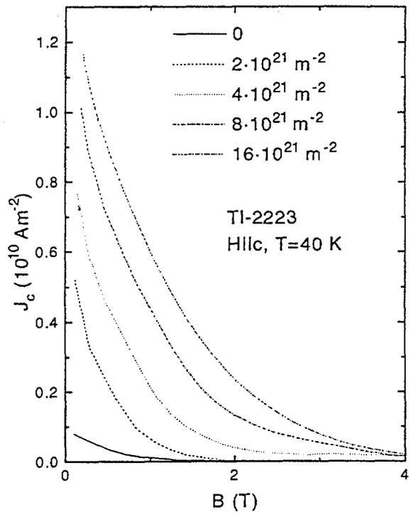
Fig. 2.  $J_c$  in a TI-2223 single crystal irradiated to different fluences.
