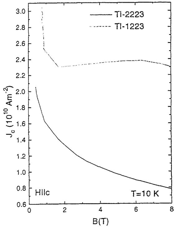
Fig. 1. Comparison of  $J_c$  at 10 K in TI-2223 and TI-1223 single crystals.
