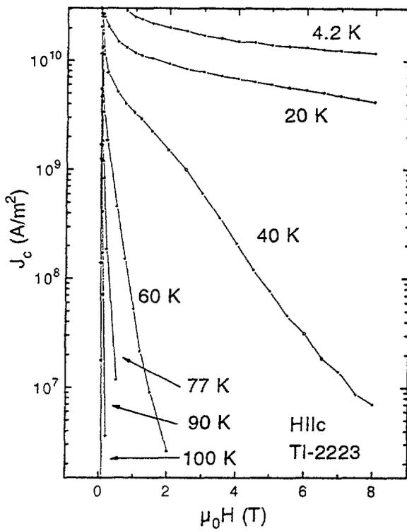
Fig. 3.  $J_c$  of a TI-2223 film.
