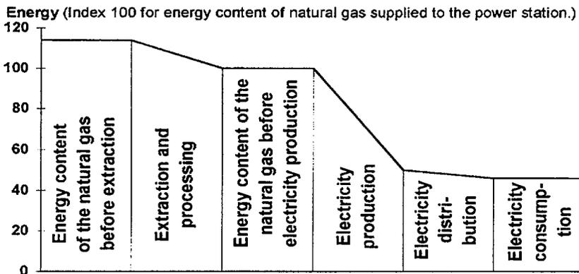
Combined heat and power production is considerably more energy efficient. The loss in producing both electricity and heating is only 10-15%. From the efficiency and environmental points of view it is preferable to produce combined heat and power to generate only electricity in a condensing plant.
