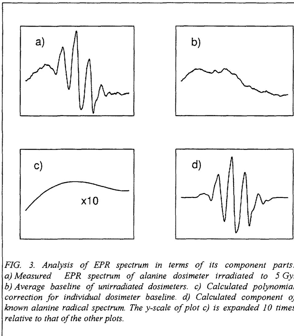
FIG. 3. Analysis of EPR spectrum in terms of its component parts: a) Measured EPR spectrum of alanine dosimeter irradiated to 5 Gy. b) Average baseline of unirradiated dosimeters. c) Calculated polynomial correction for individual dosimeter baseline. d) Calculated component of known alanine radical spectrum. The y-scale of plot c) is expanded 10 times relative to that of the other plots.
