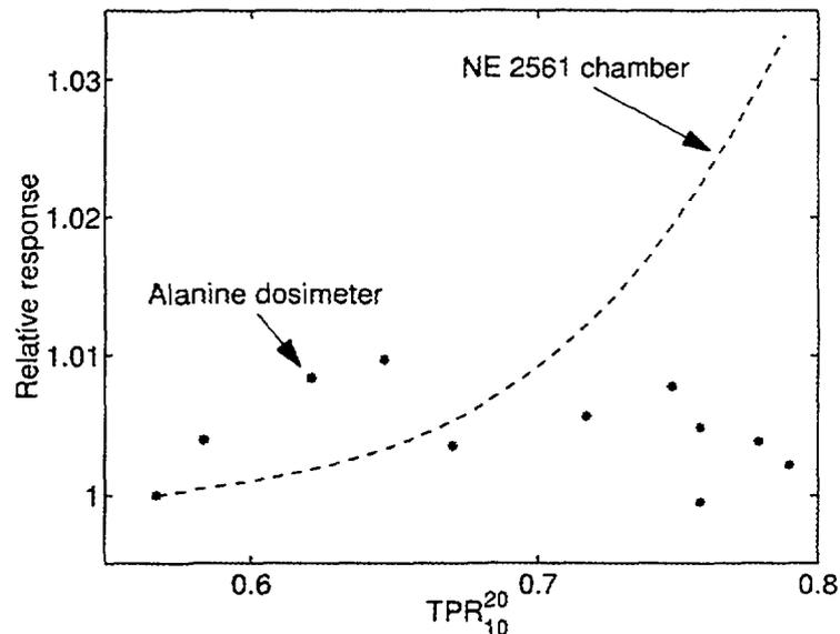
FIG. 5. Relative response of alanine dosimeters and ionisation chambers in high energy photon beams.
