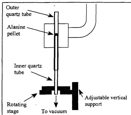
FIG. 2. Schematic diagram of system for holding alanine pellets in EPR cavity.
