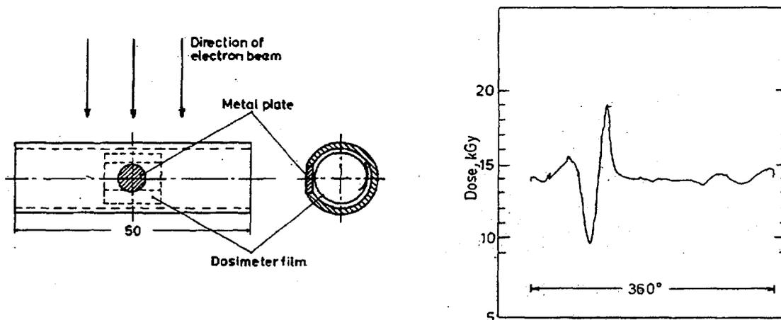
FIG. 4. The tube shown to the left was irradiated from one side with 10-MeV electrons. Dose distribution is shown to the right. 360° corresponds to a dosimeter length of 30 mm.
