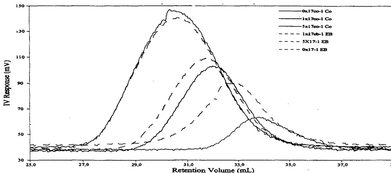
FIG. 1. The molecular weight distributions of irradiated polypropylene films irradiated by electron and gamma radiation (higher retention volume → lower molecular weight). Full lines: gamma. Dashed lines: electrons.
