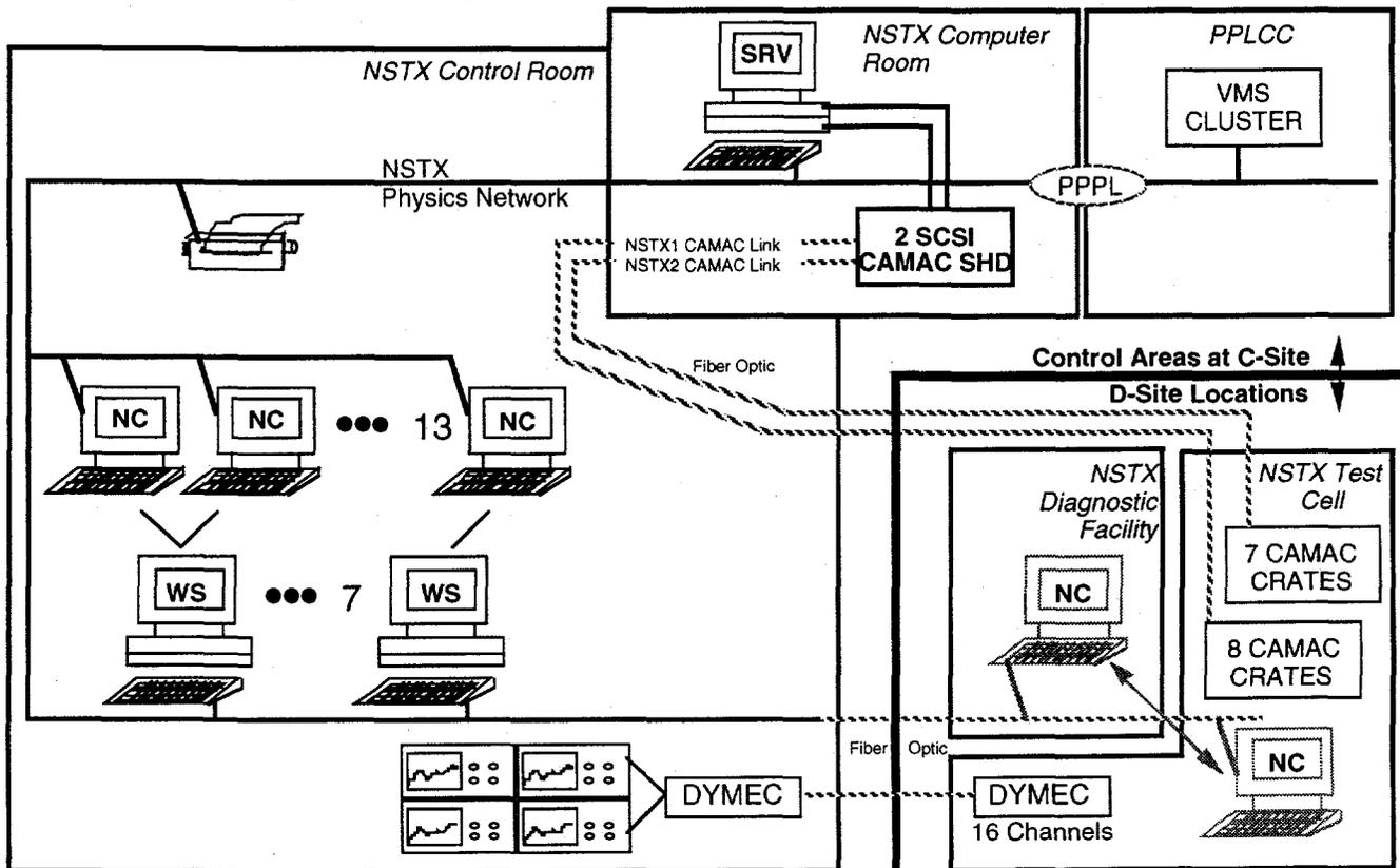
CAMAC Clock Decoder Modules will monitor the encoded timing signal and trigger timing modules in each NSTX subsystem and diagnostic.
