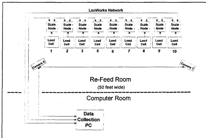
Figure 1. System Hardware block Diagram
