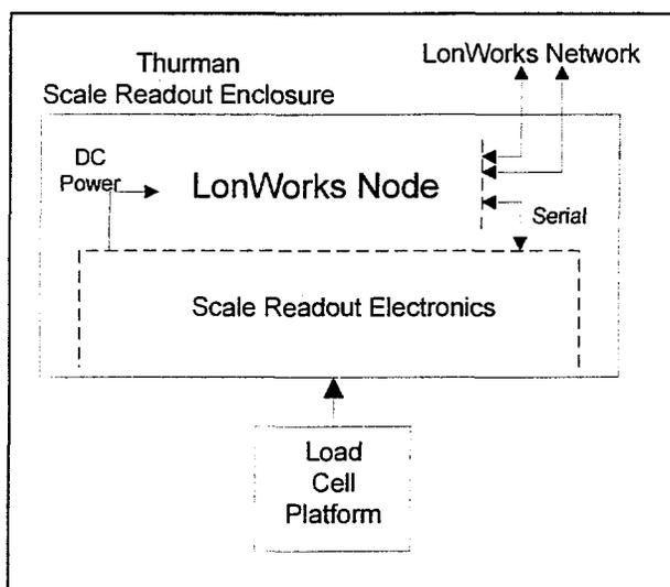
Figure 2. Modified Scale Readout Diagram
