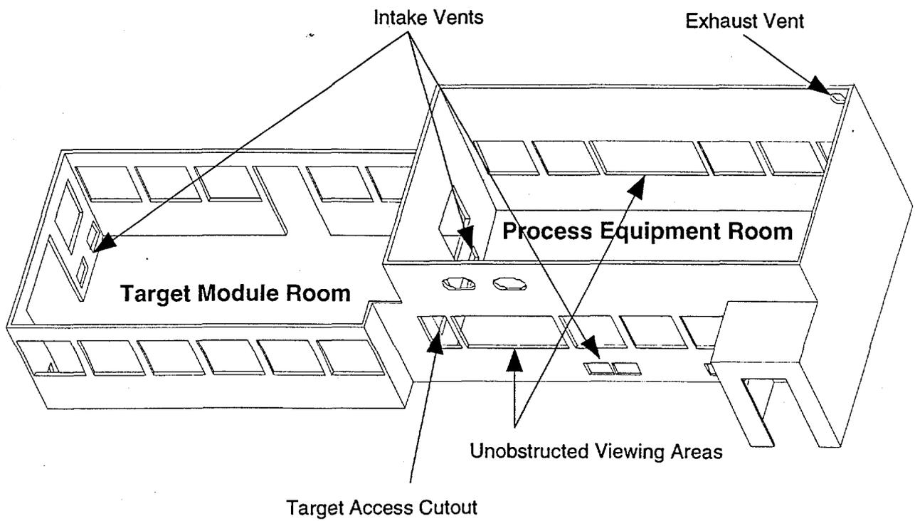
Figure 2. The TTF enclosure arrangement.
