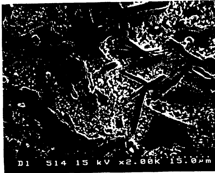
Microstructure of Shoeni 1kΩ resistor surface printed on the LTCC substrate. The sample was fired at 850°C for 30 minutes.
