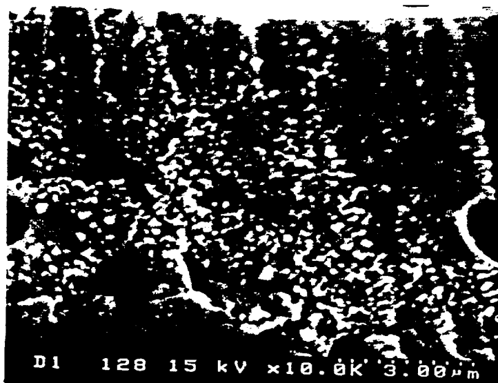
Cross-section of Shoeni 1kΩ Resistor printed of the Alumina Substrate. The Sample was Fired at 850°C for 30 Minutes.
