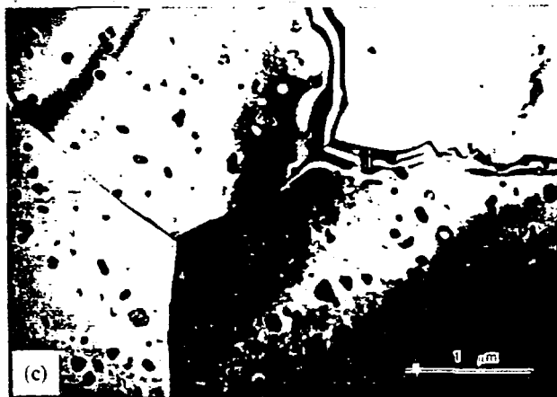
TEM micrographs of the precipitate and grain structure seen in the 7475 alloys: (a) large \eta precipitates in the as-rolled samples (b)-(d) small and stable grains and the Cr-rich particles. The pinning effect can be clearly seen in (c) and (d).
