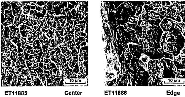
Fig. 5. SEM photograph of the center and edge of the fracture surface of the welded In 718 specimen tested in Hg.
