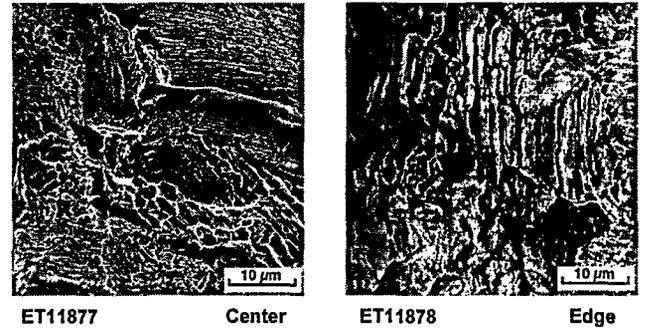
Fig. 4. SEM photographs of the center and edge of the fracture surface of the as-received In 718 specimen tested in air.
