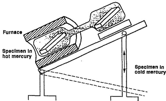
Fig. 7. Rocker apparatus used to screen for thermal gradient mass transfer.
