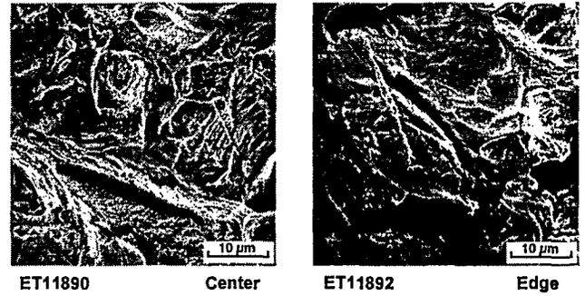
Fig. 6. SEM photographs of the center and edge of the fracture surface of the welded In 718 specimen tested in Hg-Ga.
