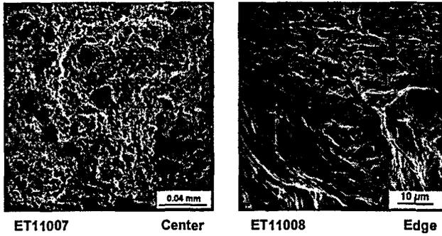
Fig. 3. SEM micrographs showing the appearance of type 316 SS tested in Hg-Ga at room temperature.
