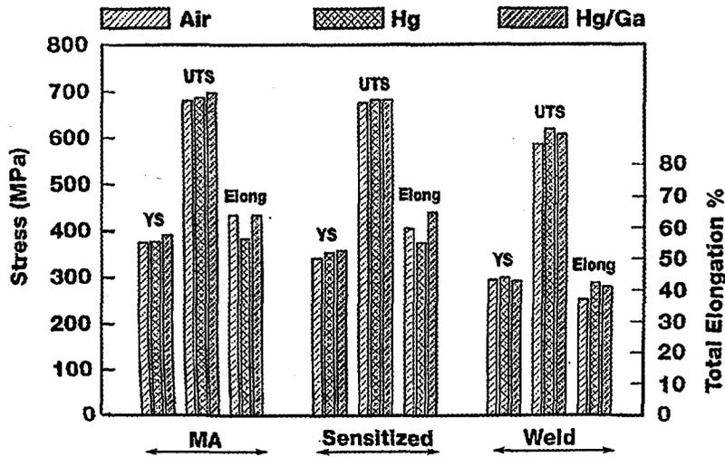
Fig. 1. Mercury or mercury-gallium did not change the room temperature tensile properties of type 316 SS in LME tests.
