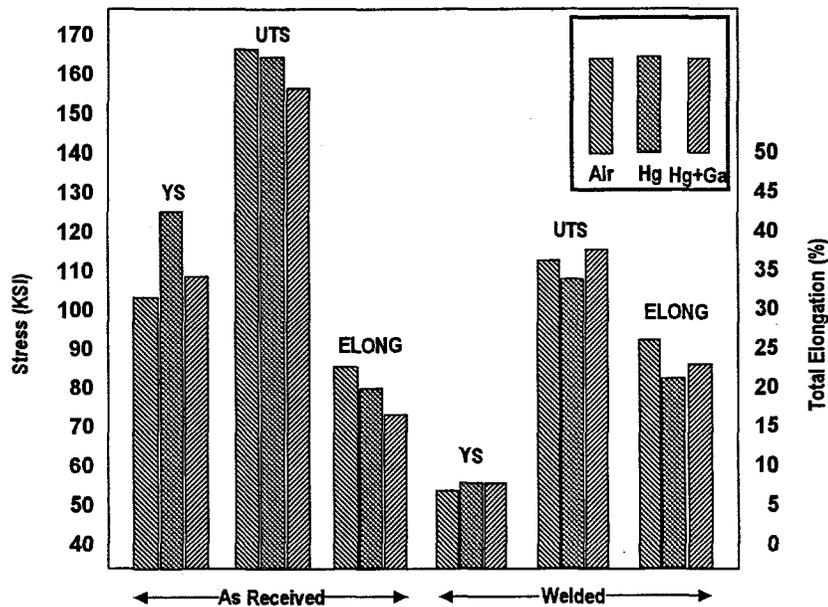
Fig. 2. Mechanical property results from constant extension rate tests for Alloy 718.
