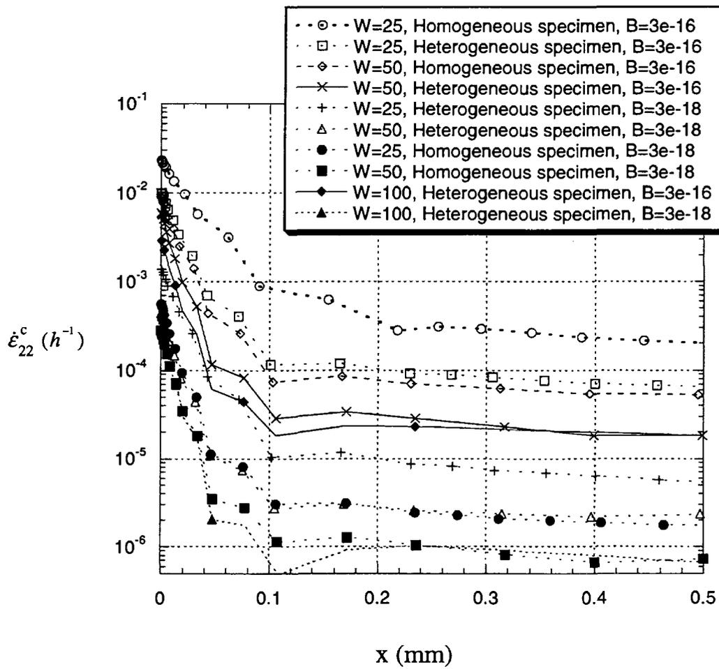
Fig. 4. The creep strain rate perpendicular to the crack plane, ahead of the crack tip, in the center of the specimens ( $z = 0$ ) for all ten CT specimen configurations.
