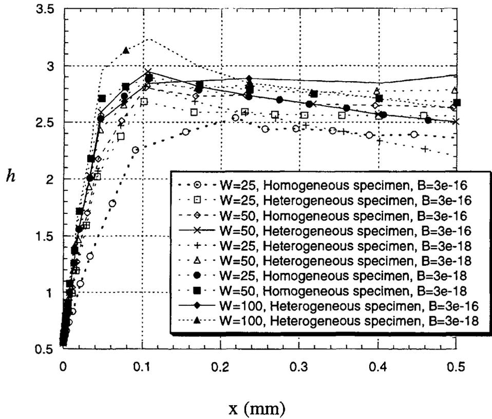
Fig. 5. The  $h$  parameter, ahead of the crack tip, in the center of the specimens ( $z = 0$ ) for all ten CT specimen configurations.
