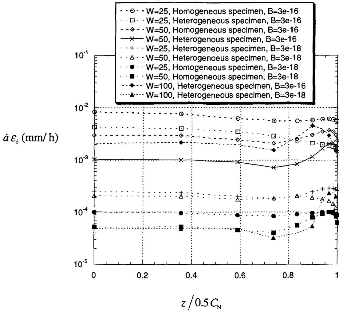
Fig. 3. The creep crack growth rate times the uni-axial creep ductility evaluated at 11 positions through the thickness of the specimens for all ten CT specimen configurations.
