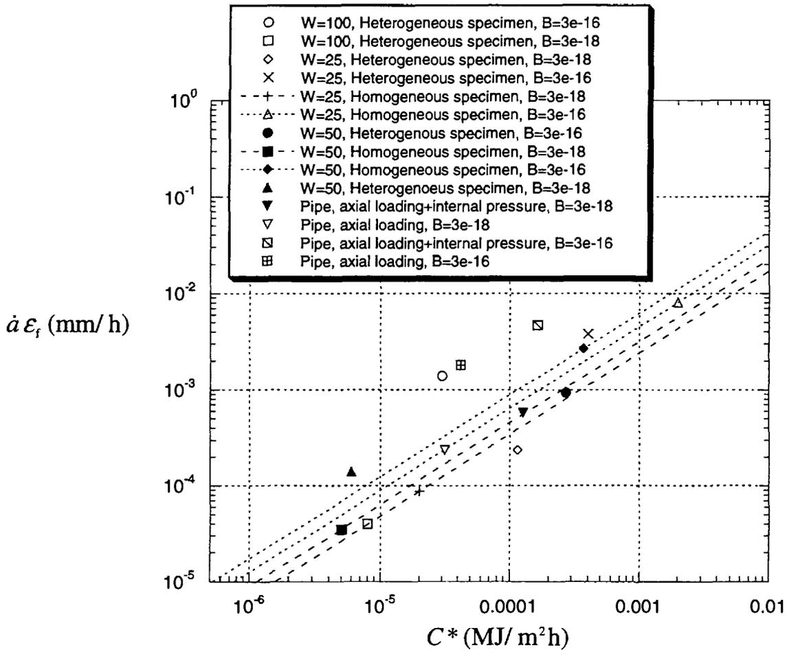
Fig. 6. The creep crack growth rate times the uni-axial creep ductility versus  $C^*$  evaluated at the center of the specimens for all ten CT specimen configurations and for the four pipe configurations.
