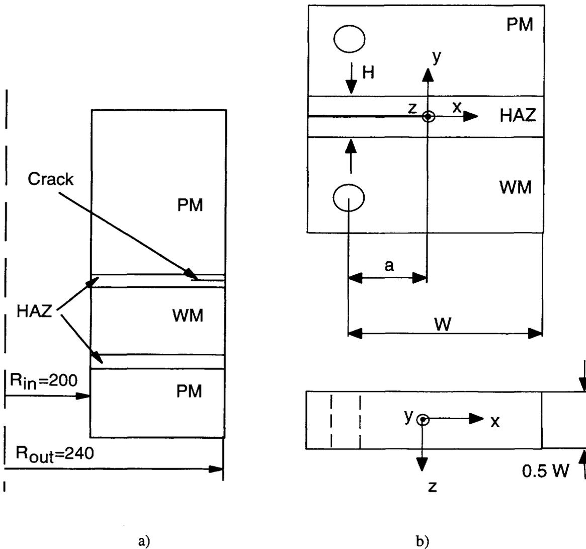
Fig. 1. a) Pipe weldment with a circumferential crack located in the HAZ [7]. b) Cross-weld CT specimen showing weldment constituents and the starter notch position. The specimens used in the finite element simulations are side grooved with a total thickness reduction of 20%. The included angle of the side groove is less than  $90^\circ$  and the root radius is less than 0.4 mm according to the ASTM E 1457 standard.
