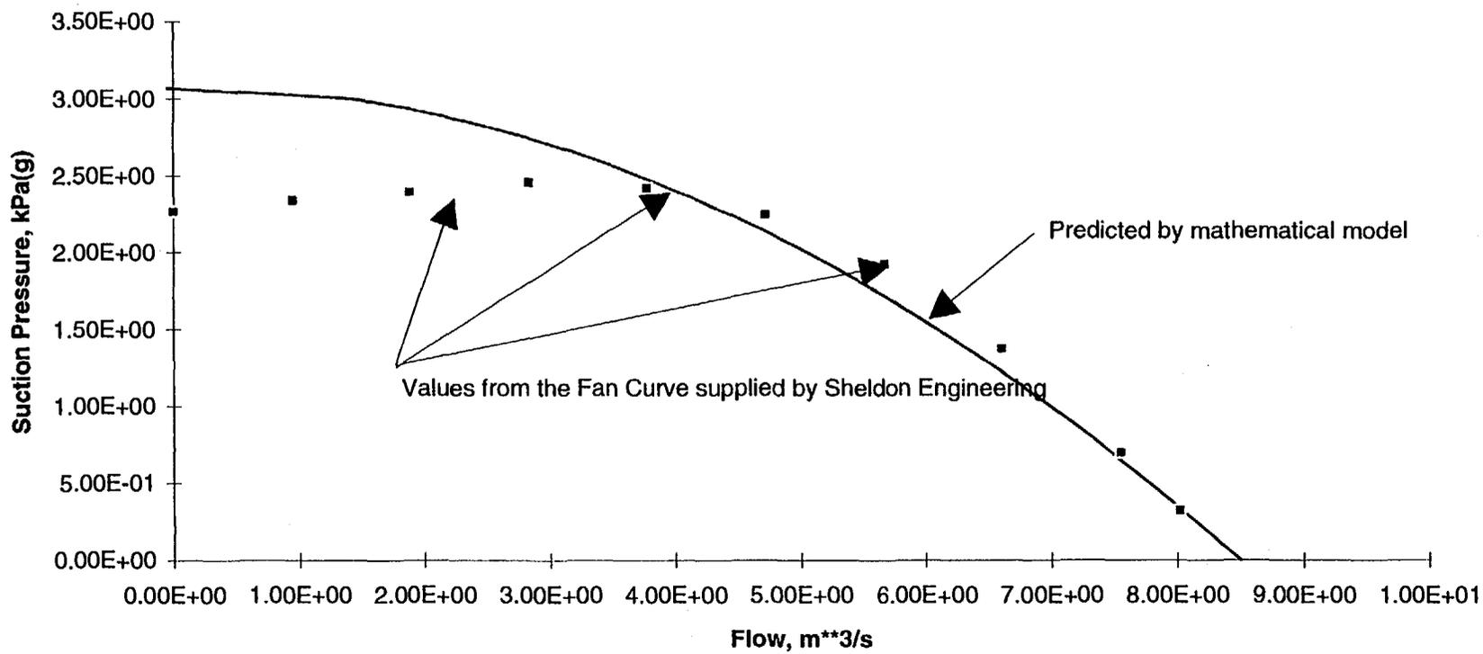
Figure-4 Predicted Fan Curve for Ventilation Outlet Fan
