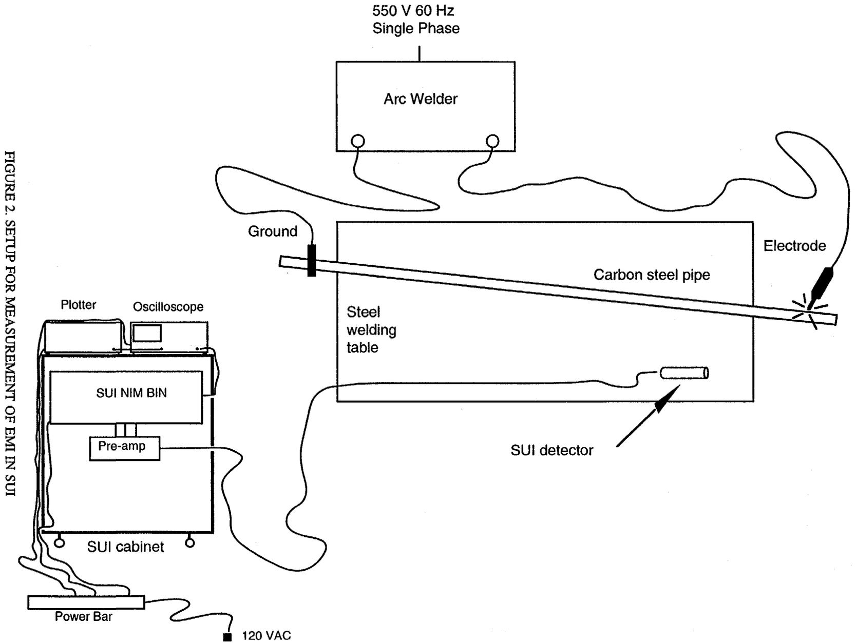
FIGURE 2. SETUP FOR MEASUREMENT OF EMI IN SUI
