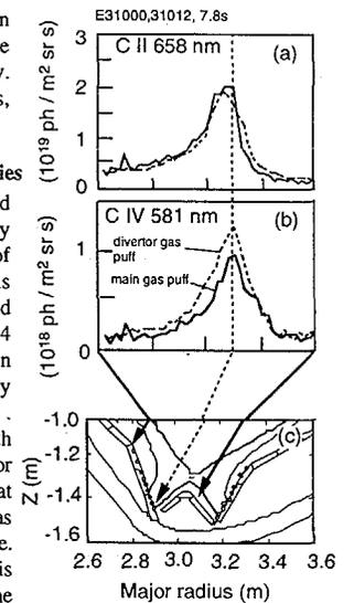
Fig. 4 Comparison of CII and CIV intensity profiles in the divertor obtained in the discharges with divertor gas puff only and main gas puff only.
