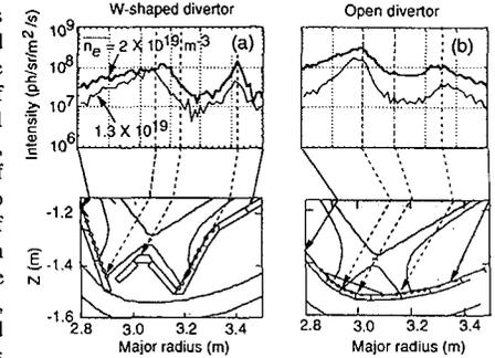
Fig. 3 Comparison of CD band intensity profiles between W-shaped divertor and open divertor
