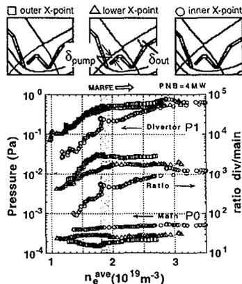
Fig. 2 Dependence of the divertor pumping slot pressure, the mid-plane pressure and pressure ratio on divertor geometry and plasma configurations.
