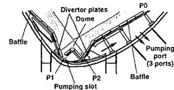
Fig. 1 Structure of W-shaped divertor
