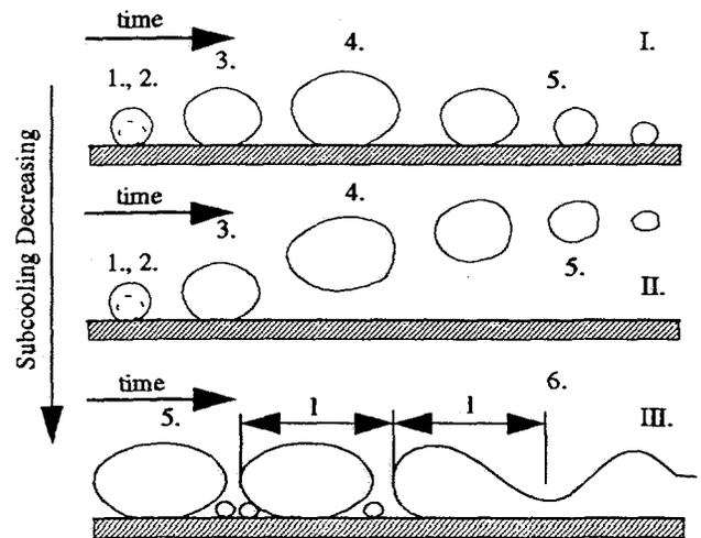
Figure 1. Vapor structures close to the heated wall in the subcooled flow boiling.
