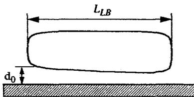
Figure 5. Schematic representation of the film thickness beneath the sliding vapor bubbles.
