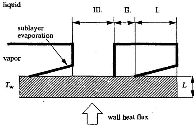
Figure 3. A schematic of structures important for the wall heat partitioning.
