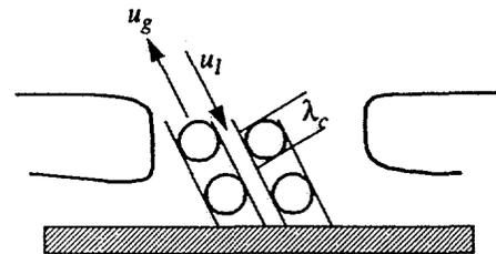
Figure 6. Schematic representation of the physics used in the calculation of the limit of liquid resupply to the sublayer.
