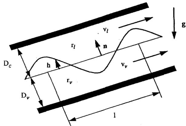
Figure 4. Confined two-dimensional wavy liquid-vapor interface.
