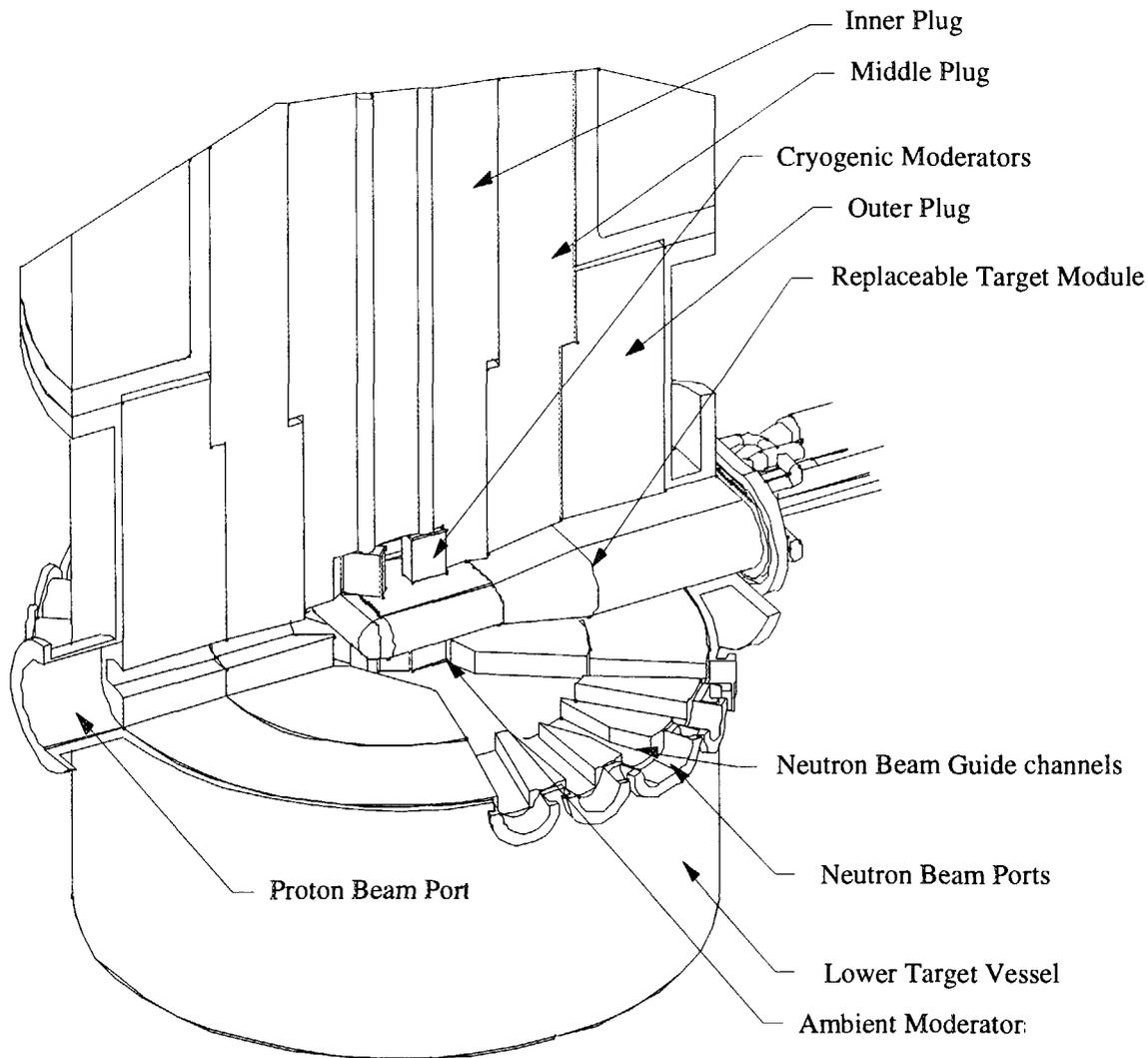
*Figure 6: Schematic of target-moderator assemblies*
