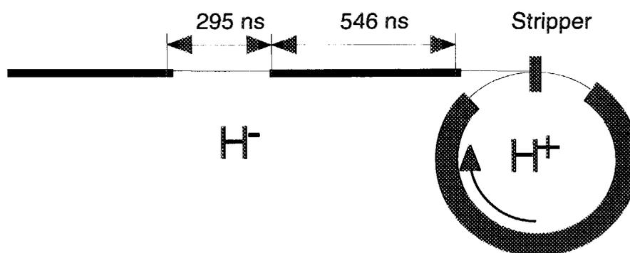
Figure 3: Schematic of beam chopping, required for minimizing beam loss during ring extraction
