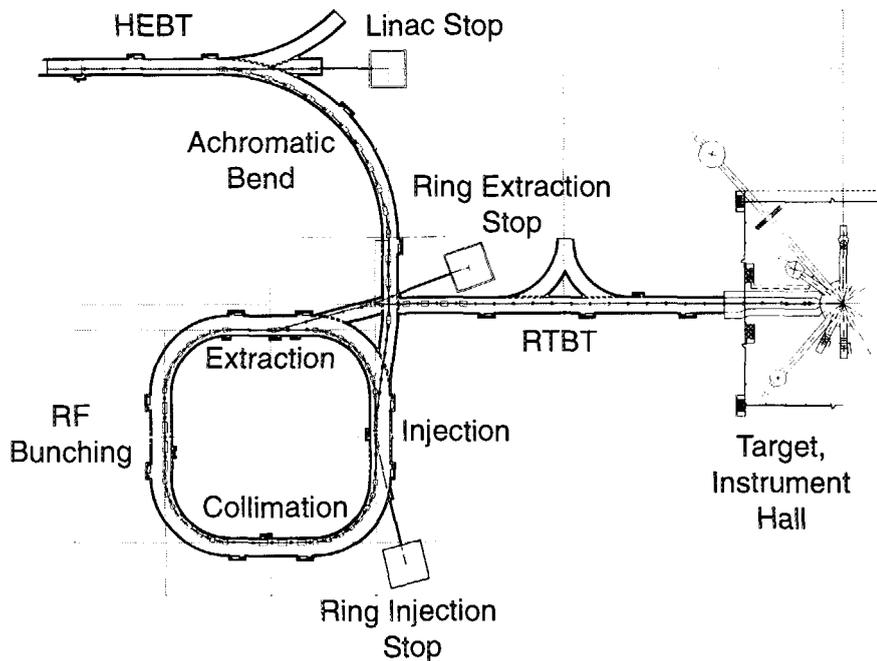
Figure 5: Transport and Accumulator Ring systems
