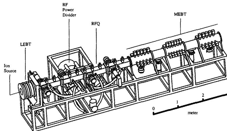
Figure 2: Front End schematic, bringing the beam to 2.5 MeV
