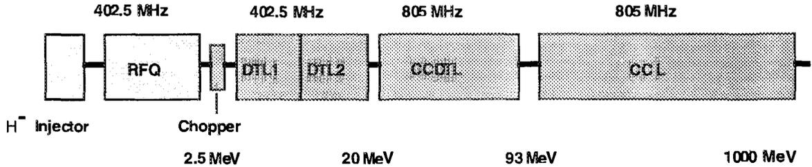
Figure 4: Schematic of linac structures that accelerate beam to 1 GeV. Lengths are not to scale: DTL is 8.7 meters long, CCDTL is 68.8 meters and CCL 417.0 meters.
