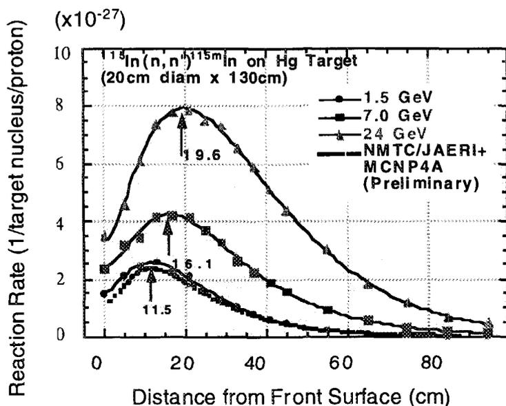
Fig. 6 Measured results of neutron emission from the mercury target
