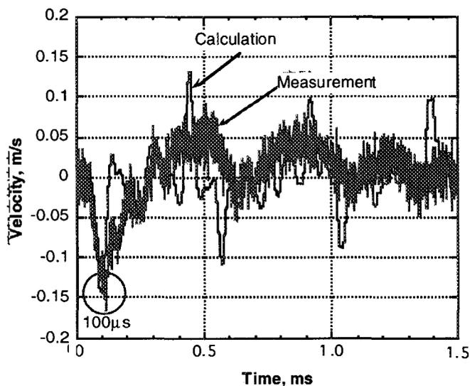
Fig.7 Velocity response measured at the container surface
