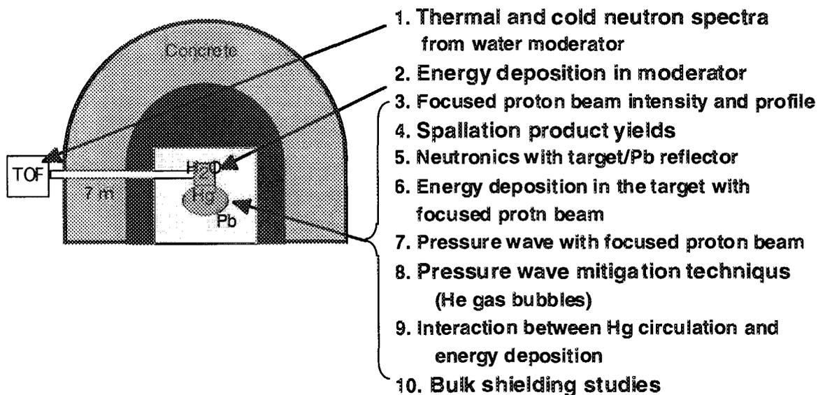
Fig. 8. Line up of the next experimental series for the ASTE collaboration
