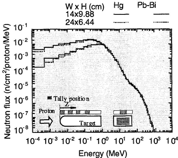
Fig.1 Comparison of neutron spectra produced by Hg and Pb-Bi targets
