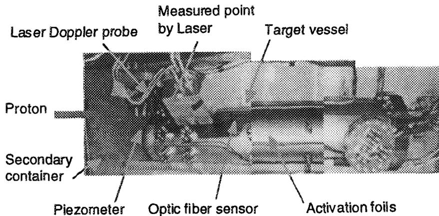
**Mercury target : 130 cm in length, 20 cm in diameter**
