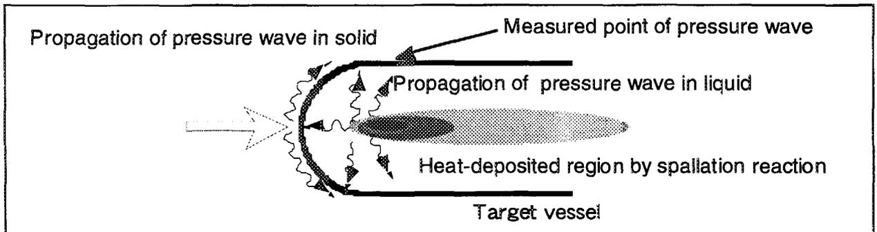
Fig.2 Pressure wave generated inside the mercury target
