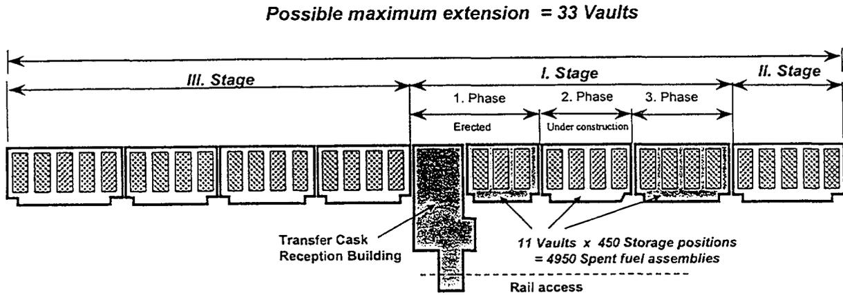
FIG. 2. Construction phases of Paks MVDS
