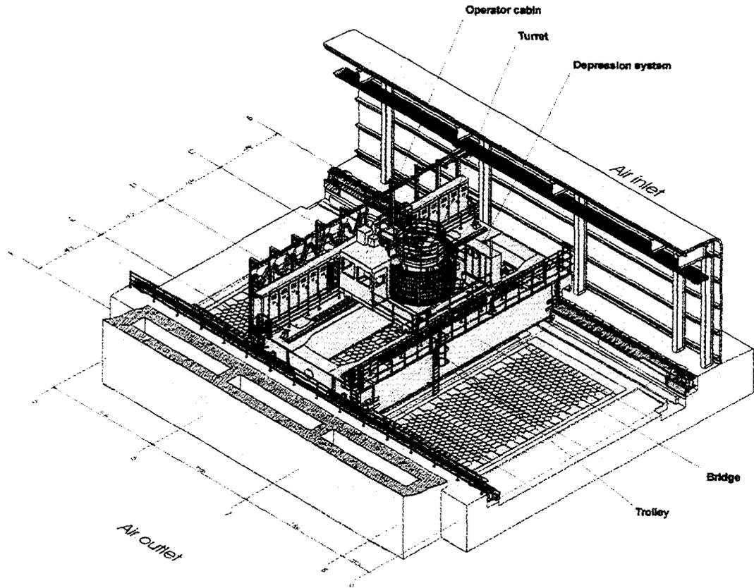
FIG. 4. Paks MVDS - Fuel handling machine
