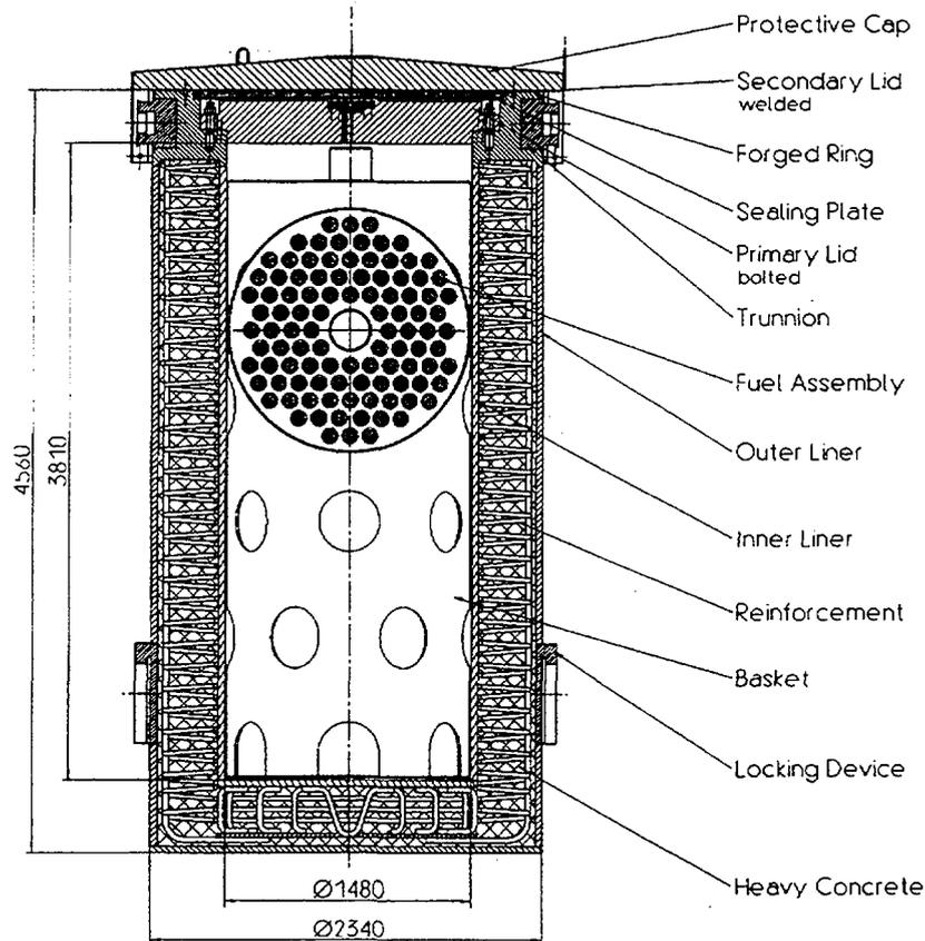
FIG. 2. CONSTOR RBMK storage cask
