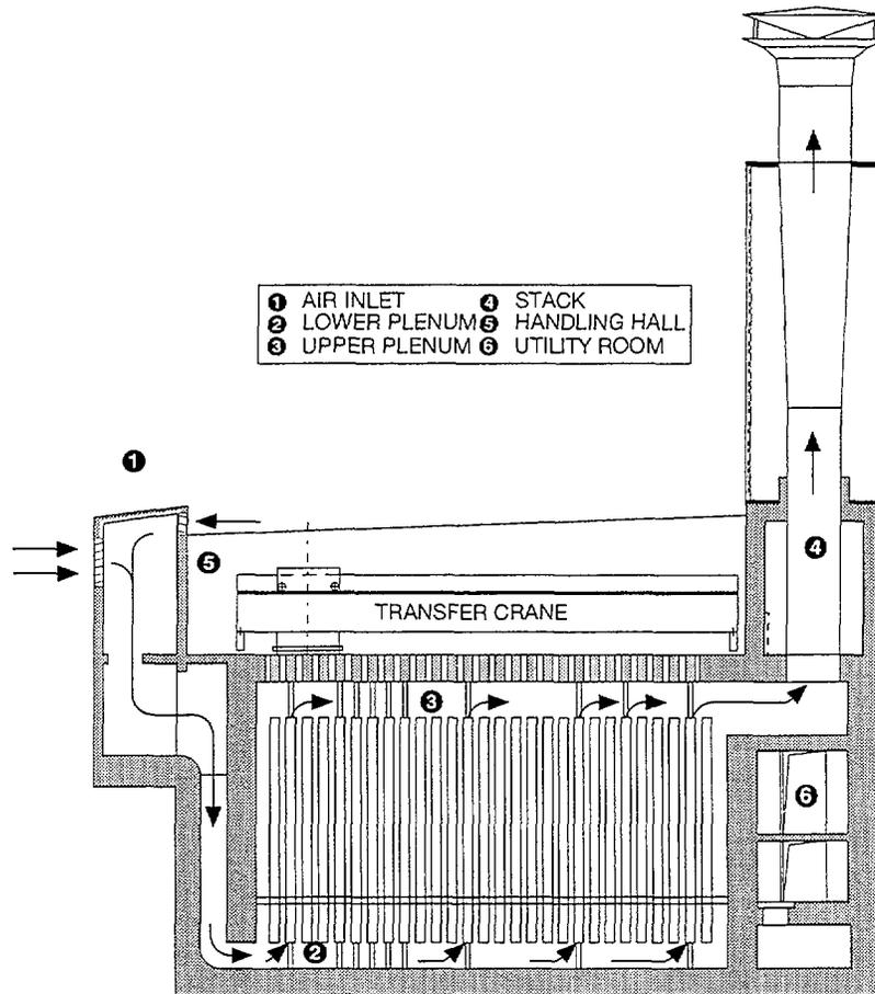
FIG. 1. Glass canister storage in EVSE facility
