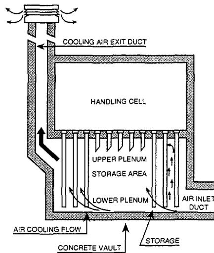
FIG. 4. Principle of passive air cooling system by natural convection
