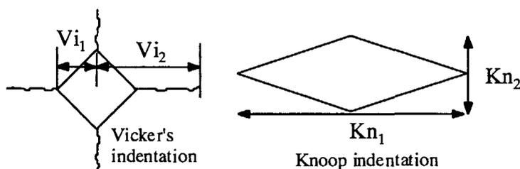
Fig. 3 Measurement of Vicker's and Knoop indentations.
