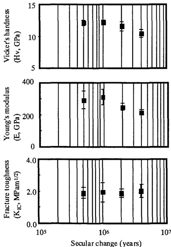
Fig. 6 Mechanical properties of Vicker's hardness (Hv), Young's modulus (E) and Fracture toughness ( $K_{IC}$ ) of "Np+U"- and "Np+U+Bi"-doped YSZ waste forms.
