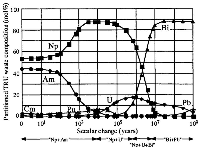
Fig. 2 Secular change of partitioned TRU waste composition ("Np-Pu" + "Am-Cm" fraction) by disintegration.
