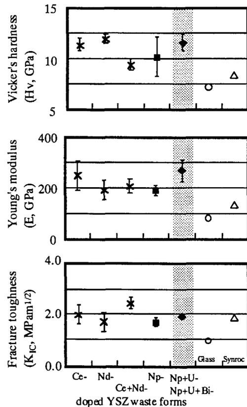
Fig. 7 Comparison of mechanical properties of Vicker's hardness, Young's modulus and fracture toughness of "Np+U"- and "Np+U+Bi"-doped YSZ waste forms with those of Ce- and/or Nd-doped YSZ waste forms, and those of a glass and Synroc waste forms.
