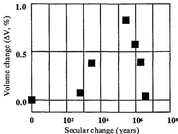
Fig. 5 Volume change of "Np+Am"-, "Np+U"- and "Np+U+Bi"-doped YSZ waste forms by the secular change of the partitioned TRU waste composition by disintegration.
