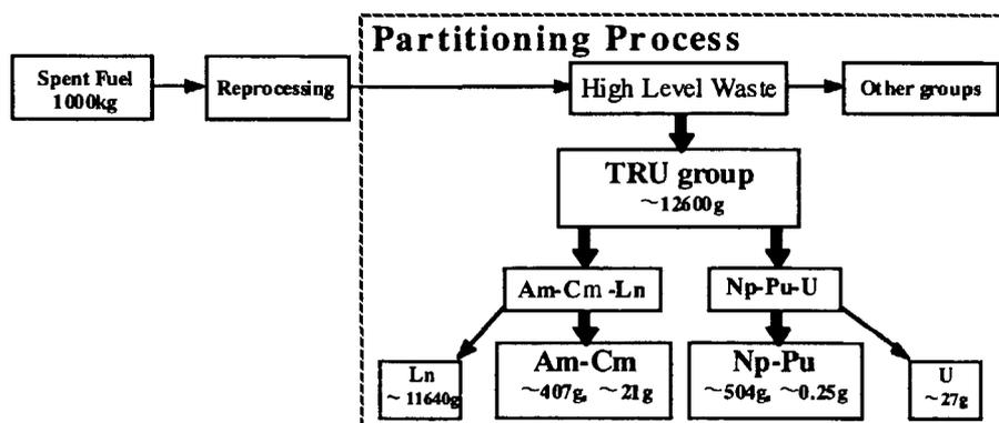
Fig. 1 Flow of TRU nuclides from spent fuel to the products in a partitioning process.
