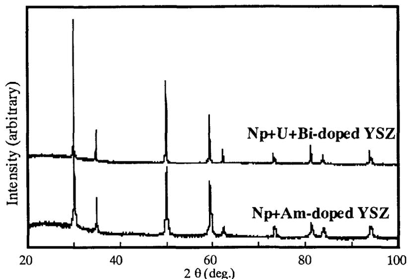
Fig. 4 XRD patterns of the initial Np+Am-doped YSZ waste form and a "Np+U+Bi"-doped YSZ waste form (sample No.7).
