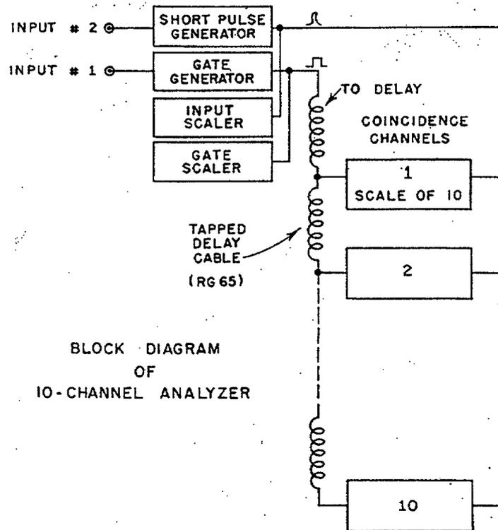
Figure 13: Block Diagram of the 10-Channel Analyzer Used by Orndorff (1957)
