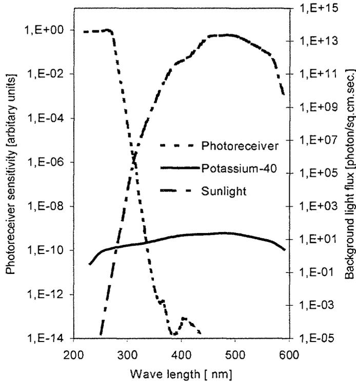
Fig.2 Spectral characteristics of photoreceiver and underwater light background.
