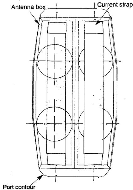
**FIGURE 1.** Front view of two-strap ion cyclotron antenna.
