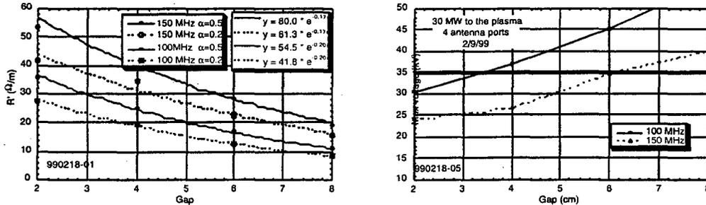
**FIGURE 3.**  $R'$  vs. gap for 100 and 150 MHz (left), and maximum voltage required to deliver 30 MW to the plasma vs. gap (right). Inter-strap phasing is  $\pi$ .
