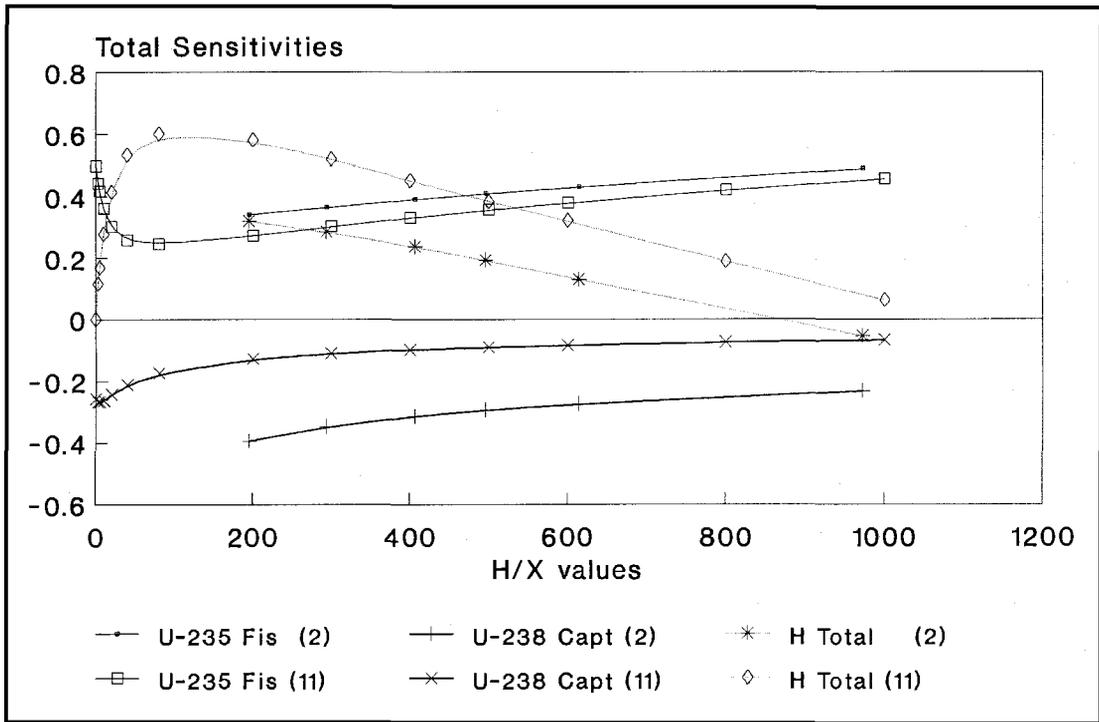
Figure 3. Total sensitivity trends with H/X for U(2)F<sub>4</sub> and U(11)O<sub>2</sub> systems.
