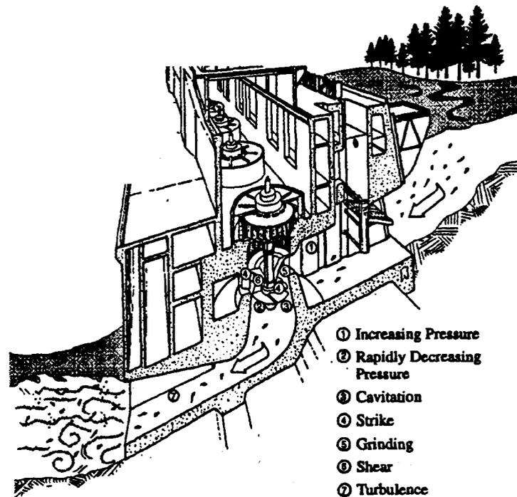
Figure 3. Locations within a hydroelectric turbine at which particular injury mechanisms may be most severe. From Čada *et al* (1997).
