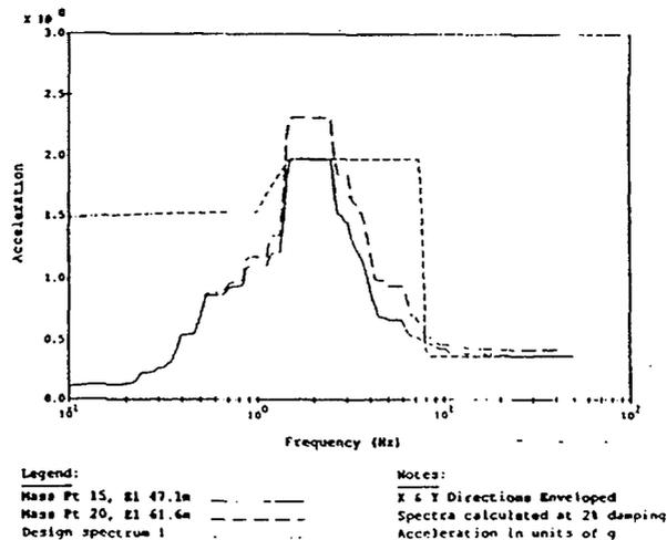
Figure 13: Containment building comparison of horizontal response to design spectrum 1-
