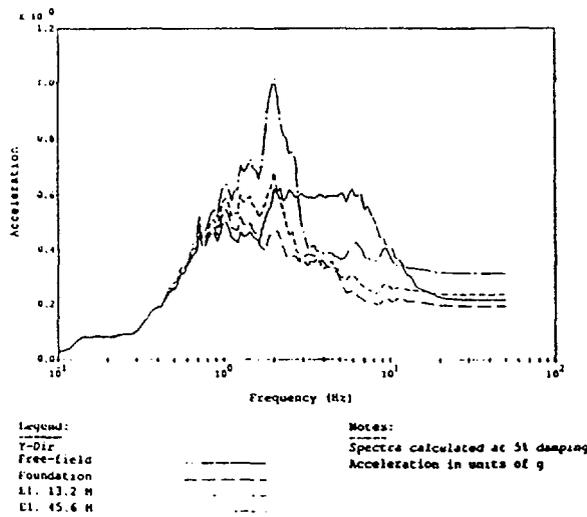
Figure 10b: Belene NPP outer building structural response layered case
