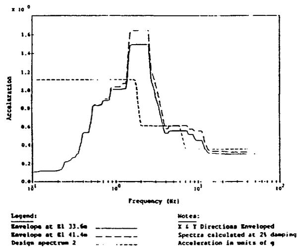
Figure 15: Outer building comparison of horizontal response to design spectrum 2
