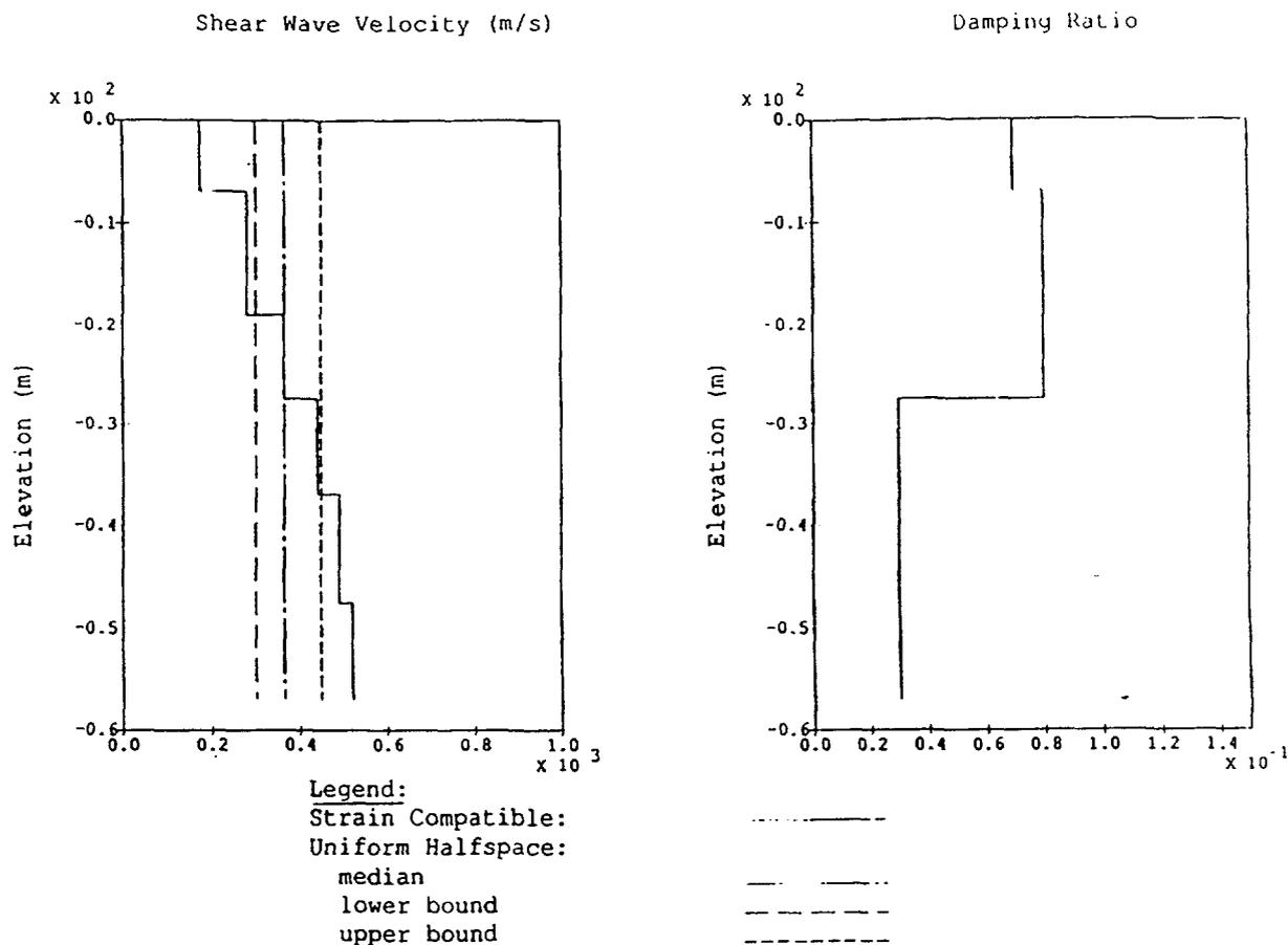
Figure 6: Variation of soil shear wave velocity and damping ratio with depth
