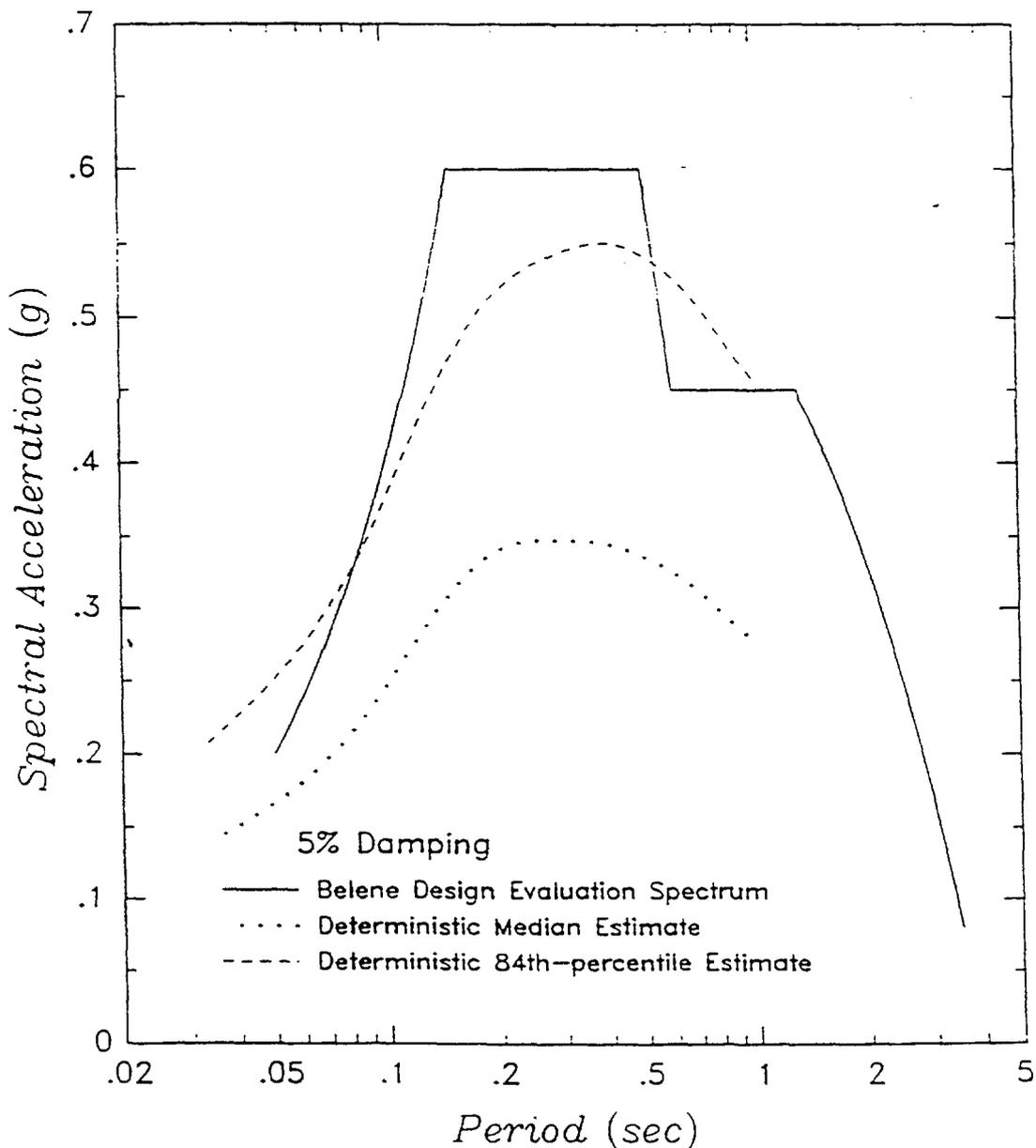
Figure 3: Comparison of the median and 84th percentile deterministic response spectra for the Vrancea source (magnitude 7.5 earthquake at an epicentral distance of 230 km) with Belene NPP design evaluation spectrum.
