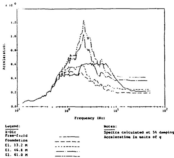
Figure 8a: Belene NPP containment building structural response layered case
