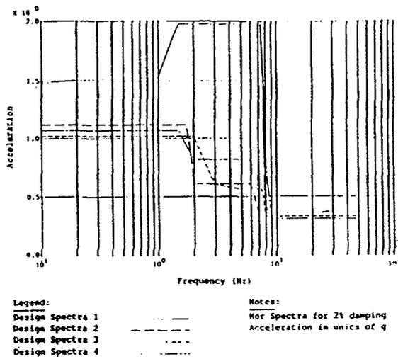
Figure 12a: Horizontal design spectra
