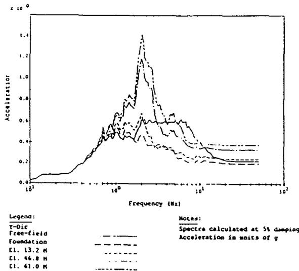
Figure 8b: Belene NPP containment building structural response layered case
