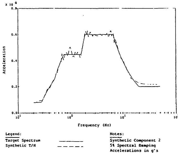
Figure 4b: Comparison of synthetic T/H's response to Belene target spectrum (Component 2)
