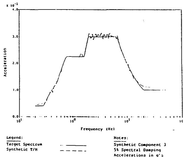
Figure 4c: Comparison of synthetic T/H's response to Belene target spectrum (Component 3)
