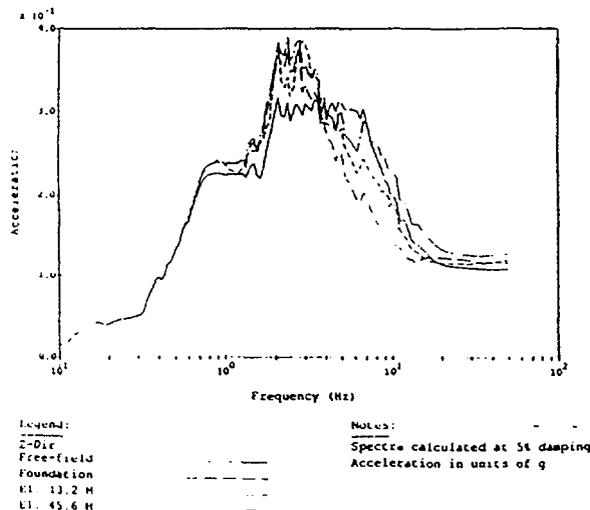
Figure 10c: Belene NPP outer building structural response layered case
