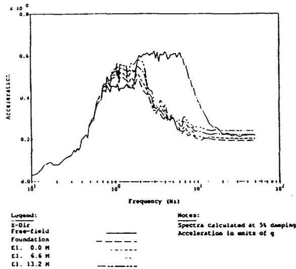
Figure 11a: Belene NPP substructure response layered case
