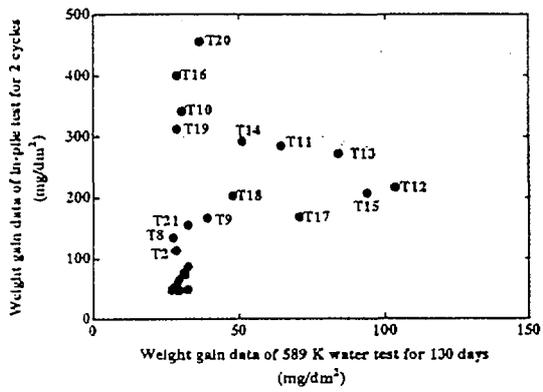
(a) In-pile test vs 589 K water test for 130 days, uniform corrosion
