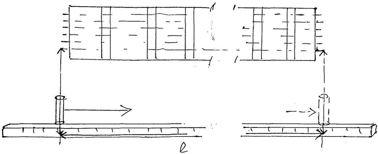
Fig. 17. Arrangement for the Length Change Determination of Fuel Assemblies
