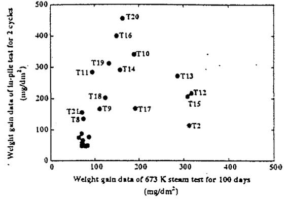
(b) In-pile test vs 673 K steam test for 100 days, uniform corrosion
