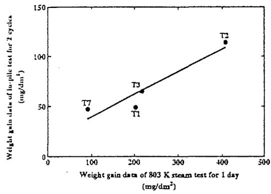
(c) In-pile test vs 803 K steam test for 1 day, nodular corrosion
