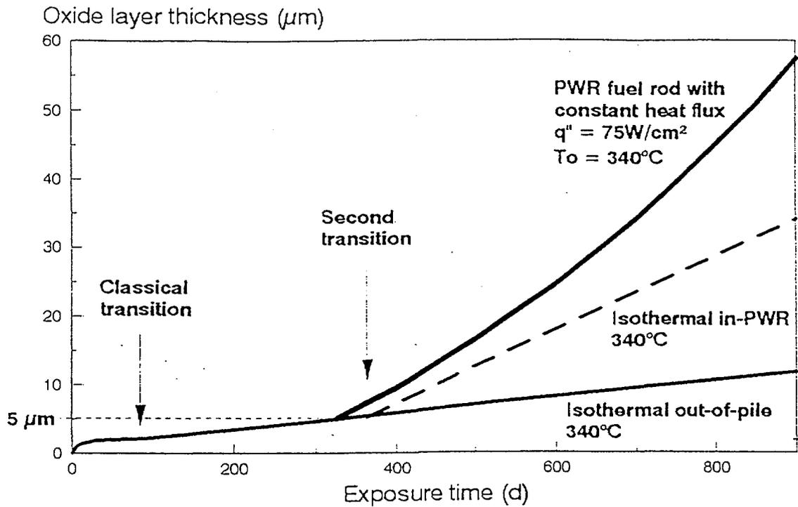
Fig. 1 Inpile and outpile Oxide Scale Growth
