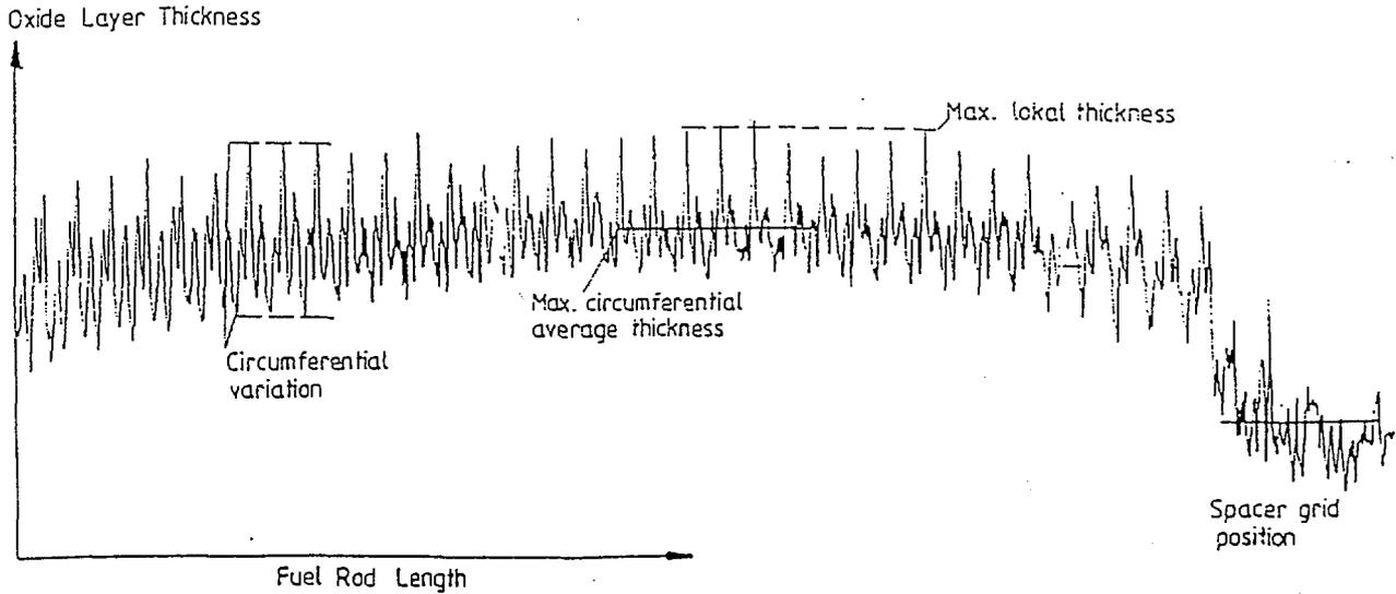
Detail A: Spiral Oxide Thickness Trace
