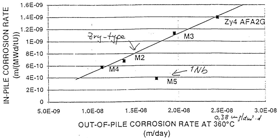
Fig. 2 Comparison of inpile and outpile Test Results
