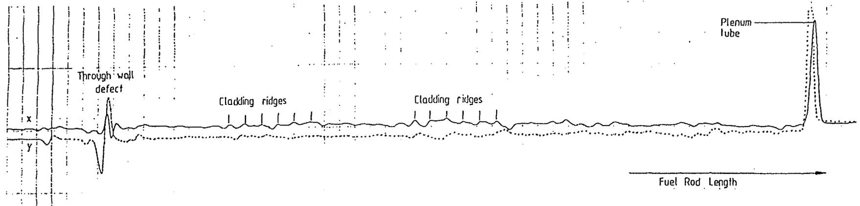
Fig. 11 EC Trace of a defective Fuel Rod
