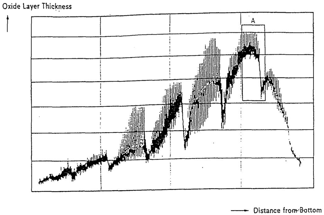
Typical Oxide Layer Thickness Profile (Spiral Trace) of a PWR Fuel Rod
