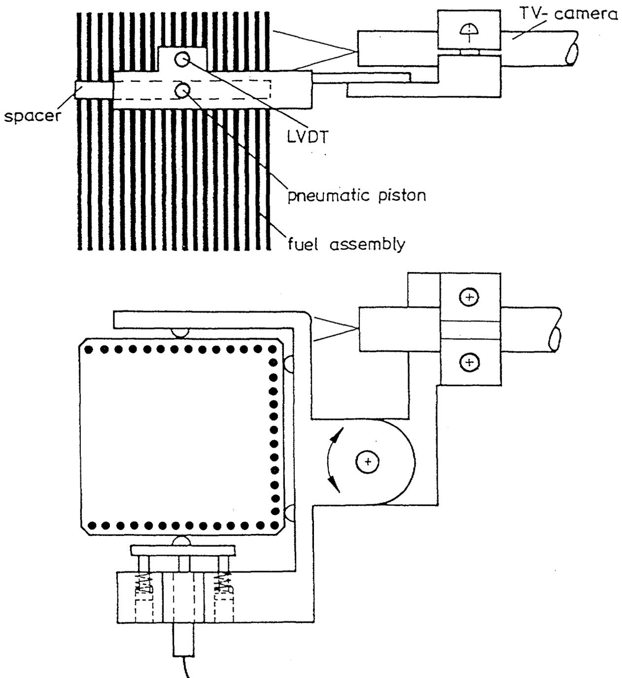
Fig. 14 Linear Variable Differential Transformer (LVDT) Device for dimensional Measurements
