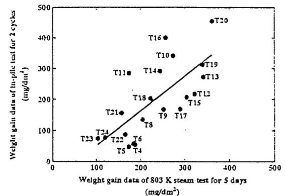
(d) In-pile test vs 803 K steam test for 5 days, uniform corrosion
