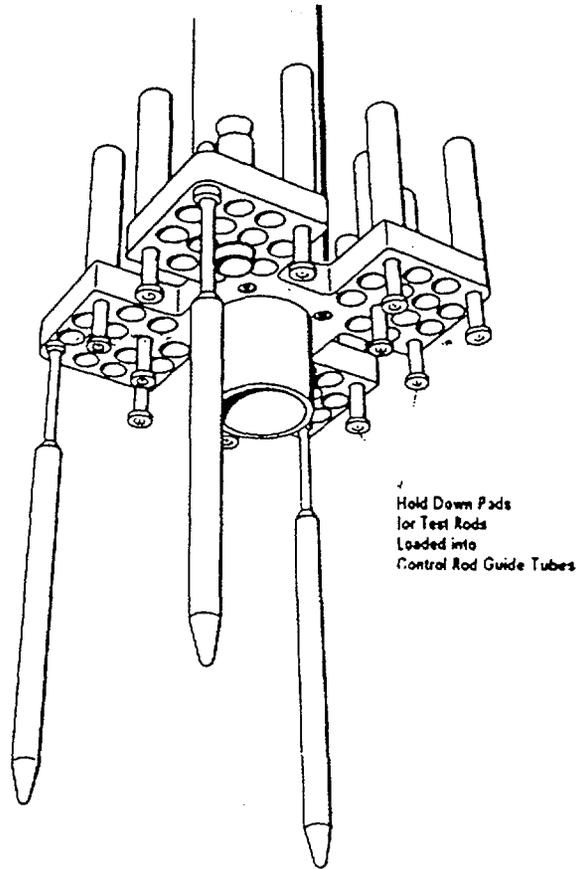
Hold Down Device for Test Rods
