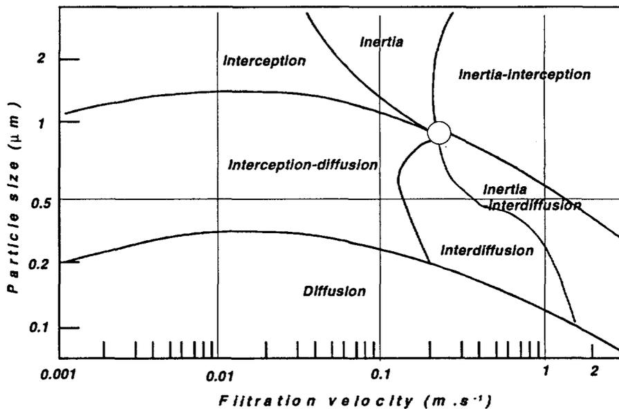
Fig. 7. Presentation of the various aerosol capture mechanisms as a function of particle size and filtration velocity (Davies, 1973)
