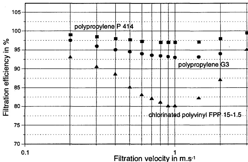
Fig. 8. Filtration efficiency of filters G3, P414 and FPP15 I-5
