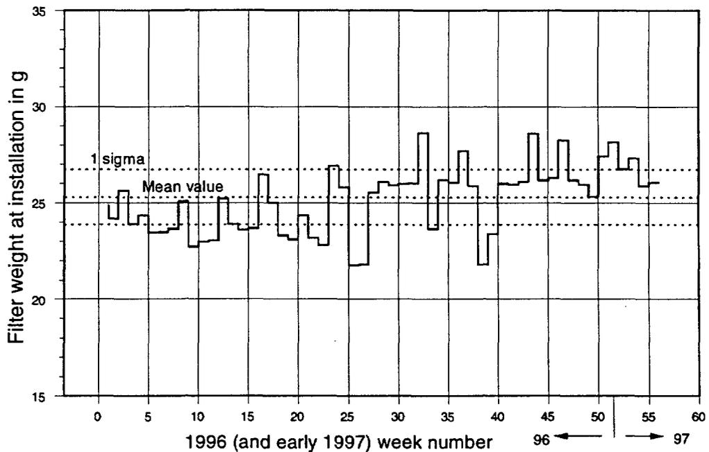
Fig. 10. Yearly variation of the weight of type G3 blank filters before installation on the ASS500 P
