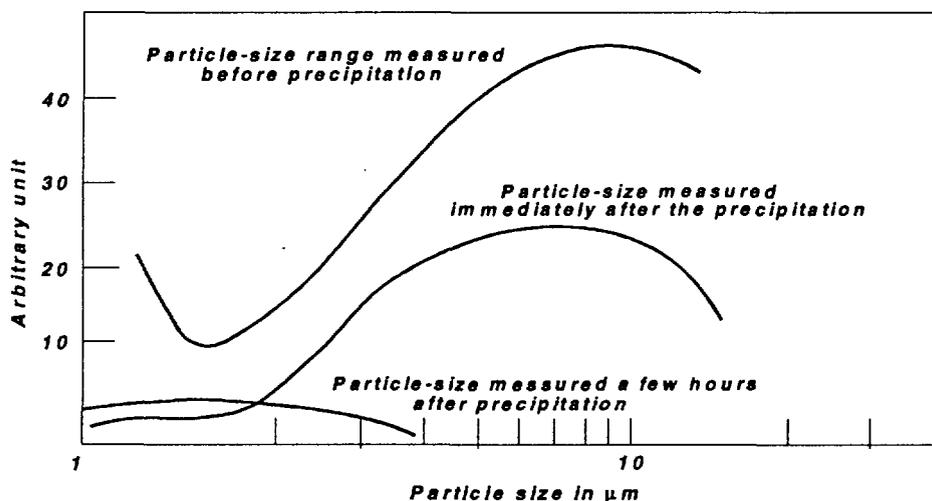
Fig. 5. Example of variation of the particle-size range of the aerosols under the effect of changing climatic conditions (cold front moving forward in the above case)
