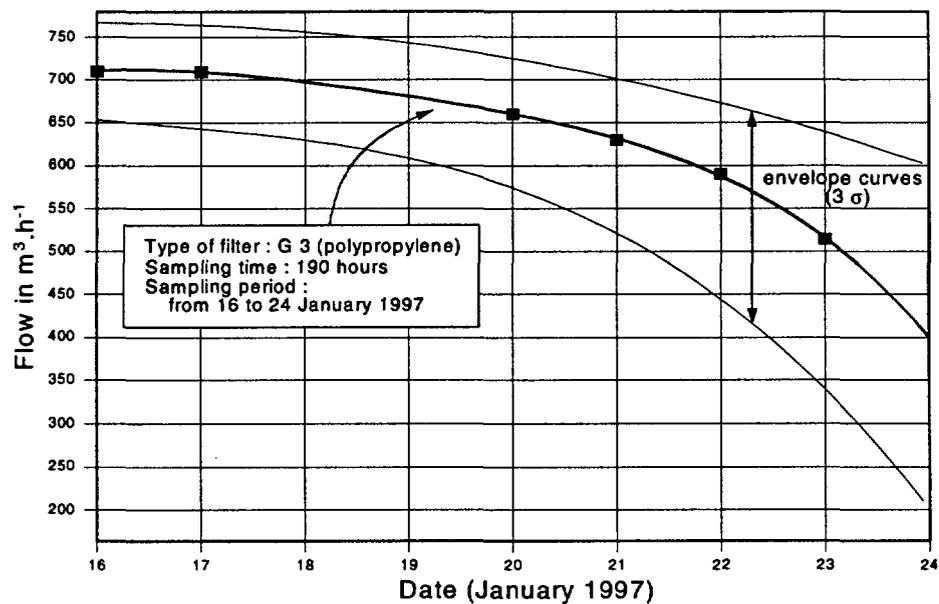
Fig. 3. Flow variation of the ASS500 P over a one-week sampling period.
