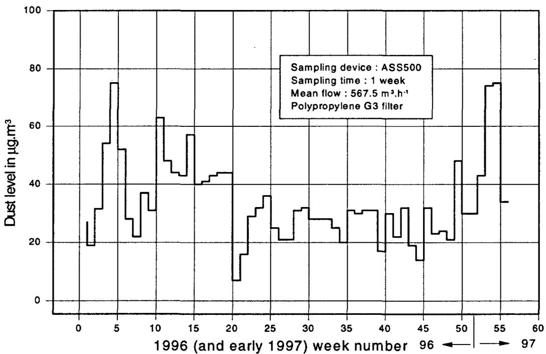
Fig. 14. Evolution of dust level (ASS500 P : 1 sampling week)
