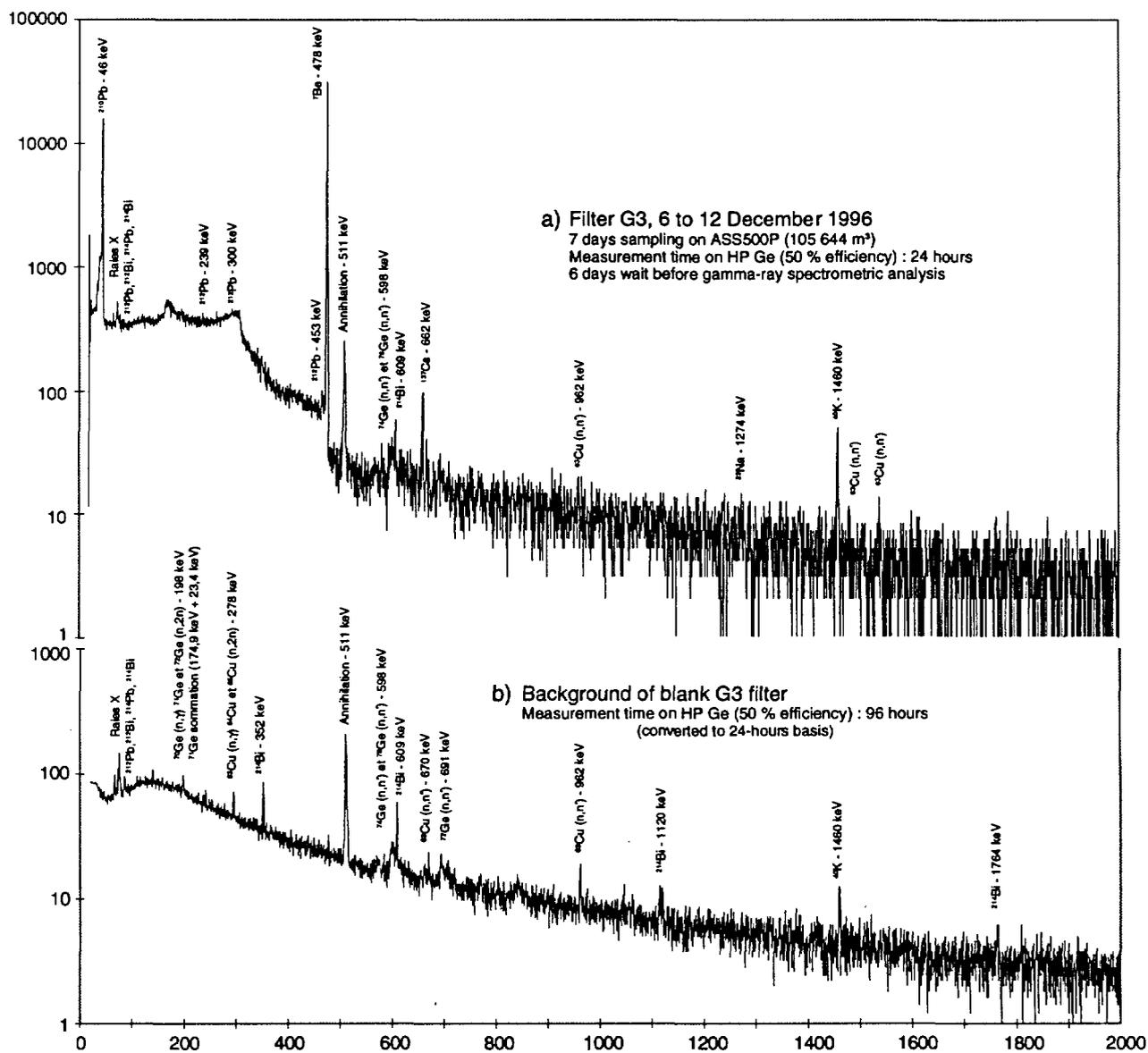
Fig. 11. a) gamma-ray spectrum of a G3 filter (7 days sampling,  $106\,000\text{ m}^3$  of filtered air sampled). b) gamma-ray spectrum of a blank filter
