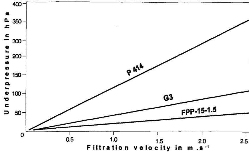
Fig. 9. Underpressure of filters G3, P414 and FPP 15 1-5
