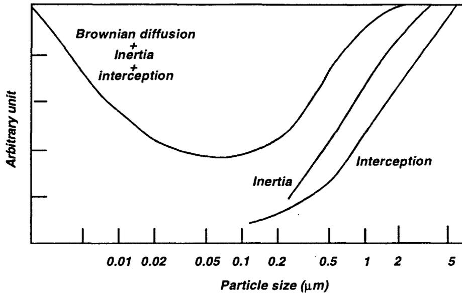
Fig. 6. Presentation of the various aerosol capture mechanisms as a function of particle size (Davies, 1973)
