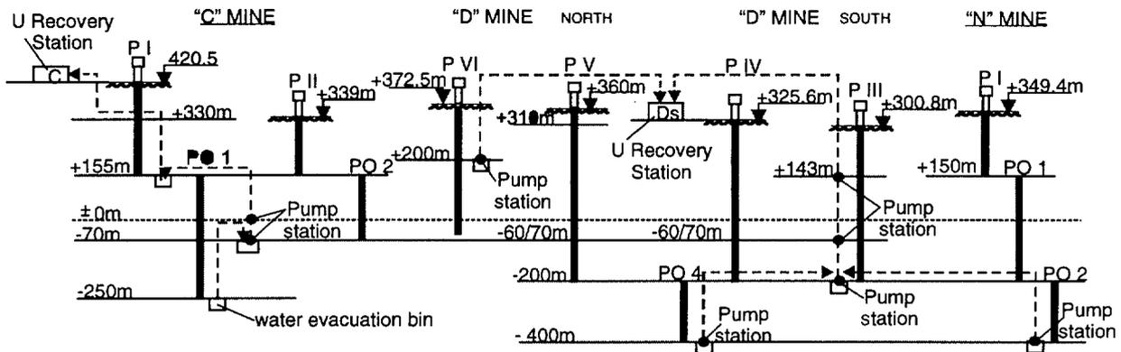
Figure 1. The diagram of opening works - underground waters evacuation system
