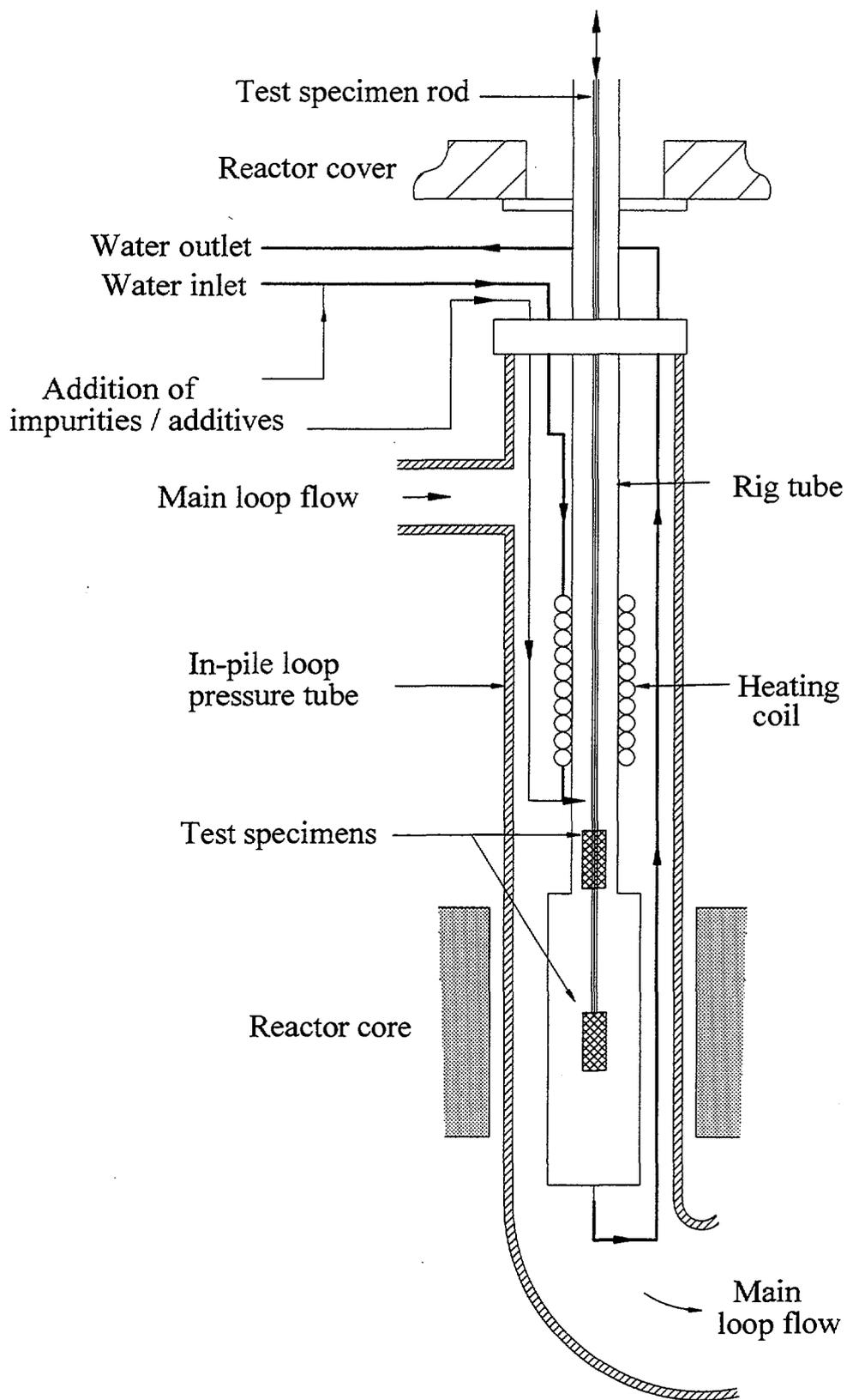
Figure 3. The in-core part of the INCA loop.
