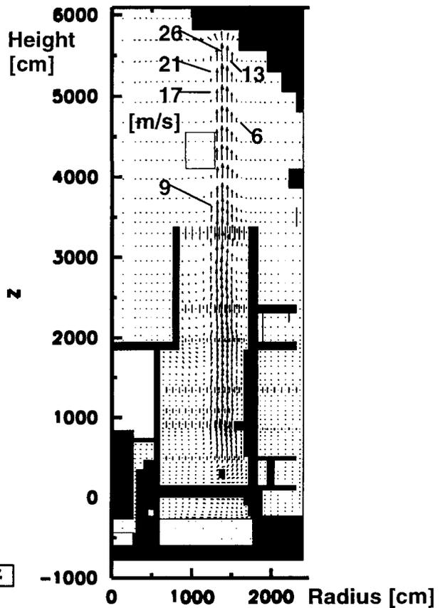
Fig. 3 : EPR; LOOP scenario with igniters 2D-velocity field at the time of maximal hydrogen release
