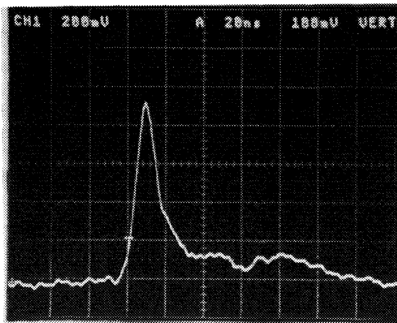
Figure 10. Temporal profile of second harmonics of GSGG laser.
