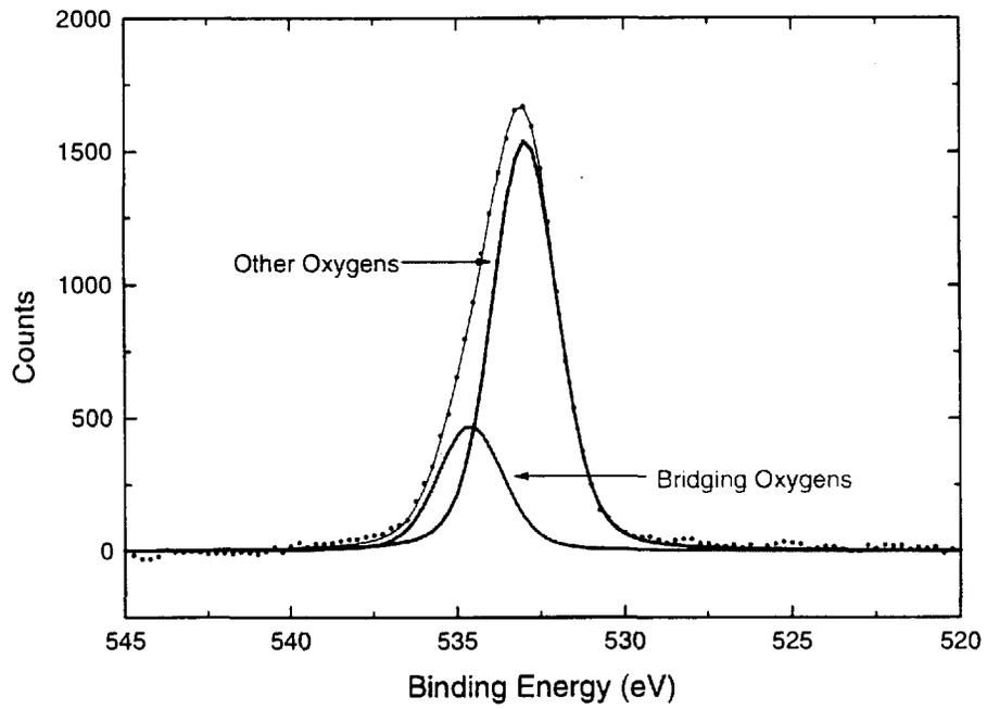
**Figure 8.** O 1s XPS spectrum for an iron phosphate glass whose batch composition was 31Fe<sub>3</sub>O<sub>4</sub>-69P<sub>2</sub>O<sub>5</sub> (mol%).
