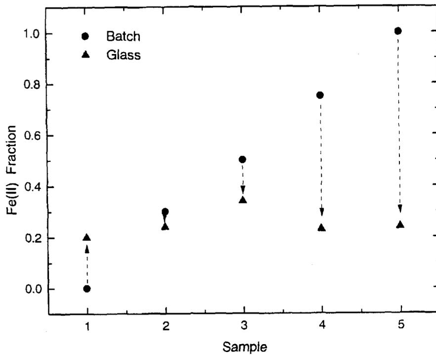
**Figure 3.** Fraction of Fe(II) in air melted glasses(A) and their batches(O). Fe/P ratio is 0.67 for ail glasses shown above.  $\text{FeO}$ ,  $\text{Fe}_2\text{O}_3$ ,  $\text{Fe}_3\text{O}_4$ , or  $\text{Fe}_2\text{C}_2\text{O}_4 \cdot 2\text{H}_2\text{O}$  or a combination of these iron oxides were used in the batch.
