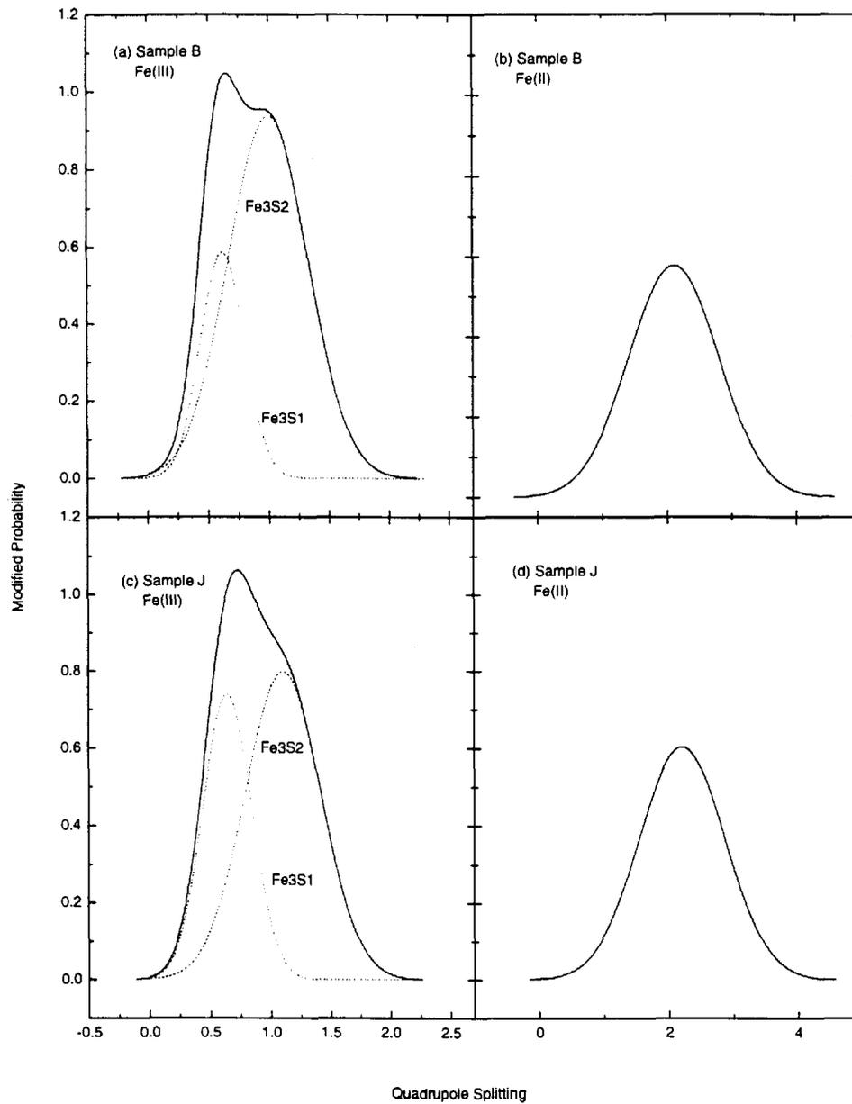
**Figure 4.** Quadrupole Splitting distributions at iron sites for two iron phosphate glasses containing 23% Fe(II) (a & b) and 40% Fe(II) (c & d).
