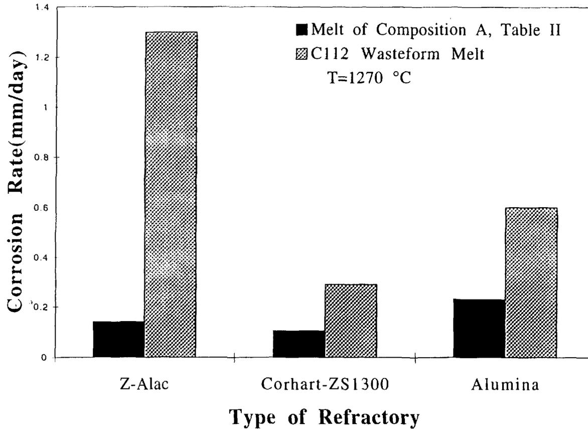
**Fig. 13.** Comparison of melt-line corrosion rates for different refractories in molten composition A and in an iron phosphate melt that contains 50 wt% of the Hanford C-112 waste. See text for melt compositions. Corrosion was measured at a melt temperature of 1270° C. The corrosion rate in the C-112 wasteform melt is consistently higher than that in melt A for all the refractories.
