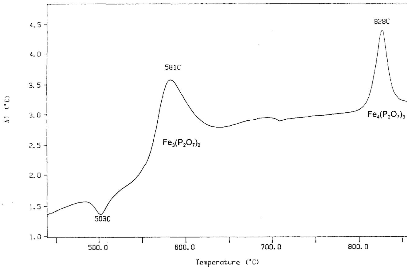
**Fig. 9.** Differential thermal analysis (DTA) for a 40Fe<sub>2</sub>O<sub>3</sub>-60P<sub>2</sub>O<sub>5</sub>, mol%, glass (glass A, Table II) at a heating rate of 10° C/min. Weight of the sample: ~40 mg; Particle size: 25-45 μm; Atmosphere: Flowing (30 cm<sup>3</sup>/min) nitrogen gas. Exothermic peaks at 581° C and 828° C correspond to the crystallization of Fe<sub>3</sub>(P<sub>2</sub>O<sub>7</sub>)<sub>2</sub> and Fe<sub>4</sub>(P<sub>2</sub>O<sub>7</sub>)<sub>3</sub>, respectively.
