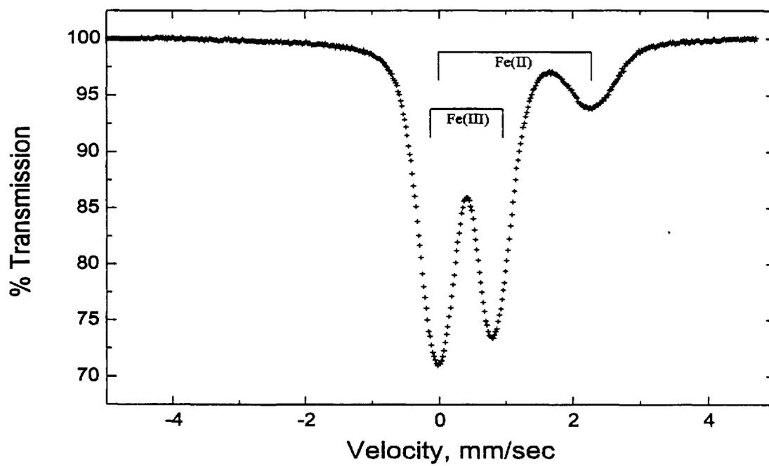
**Figure 2.** Mössbauer spectrum measured at 295 K of an iron phosphate glass of batch composition  $40\text{Fe}_2\text{O}_3\text{-}60\text{P}_2\text{O}_5$ (mol%).
