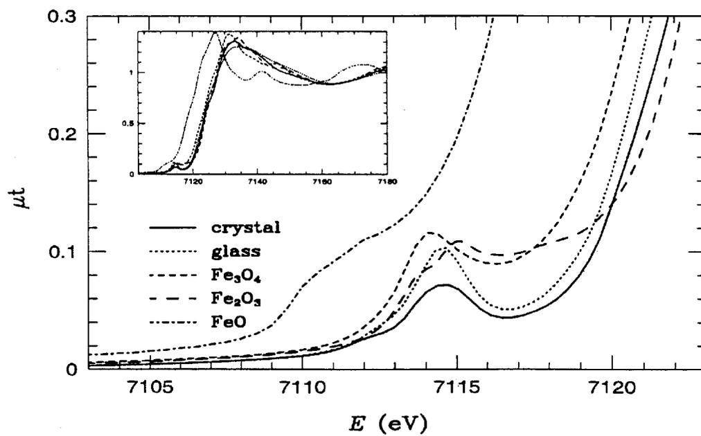
**Figure 5.** 1s-3d feature in XANES data for a glass with batch composition 31  $\text{Fe}_3\text{O}_4$ -69 $\text{P}_2\text{O}_5$  (mol%), its crystalline counterpart and several iron oxides.
