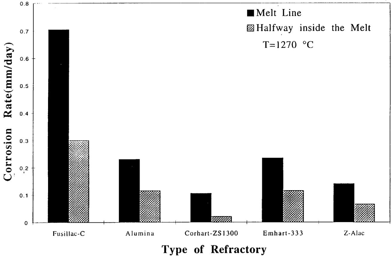
Fig. 12. Corrosion rate for different refractories rotated in molten  $40\text{Fe}_2\text{O}_3\text{-}60\text{P}_2\text{O}_5$ , mol%, Table II, at  $1270^\circ\text{C}$ . While the corrosion rate of Corhart-ZS 1300 in this melt is the lowest and that of Fusillac-C is the highest, the corrosion rates for all these refractories are considered generally low in this melt.
