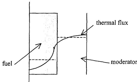
Figure: 8: Thermal flux distribution in a unit cell.
