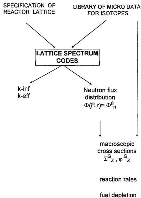
Figure 13: General diagram of the input and output of a reactor lattice code.
