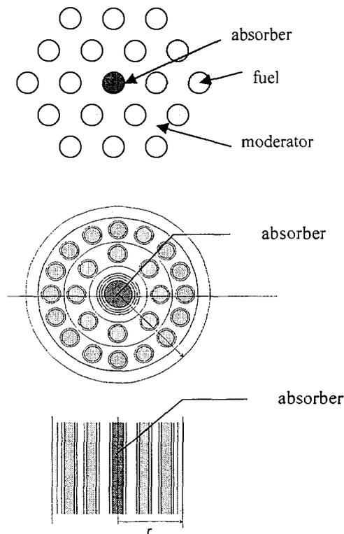
Figure 6: Possible macrocells with fuel rods and fuel plates with an absorber.
