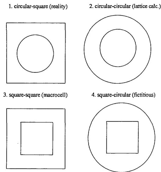
Figure 7: Possible schemes of fuel element and outer cell boundaries.
