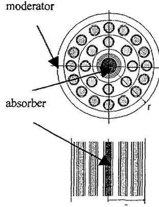
Figure 17: Model of a 'cluster' in cylindrical and plane geometry.
