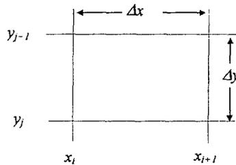
Figure 11. Spatial mesh in  $(x,y)$  geometry.
