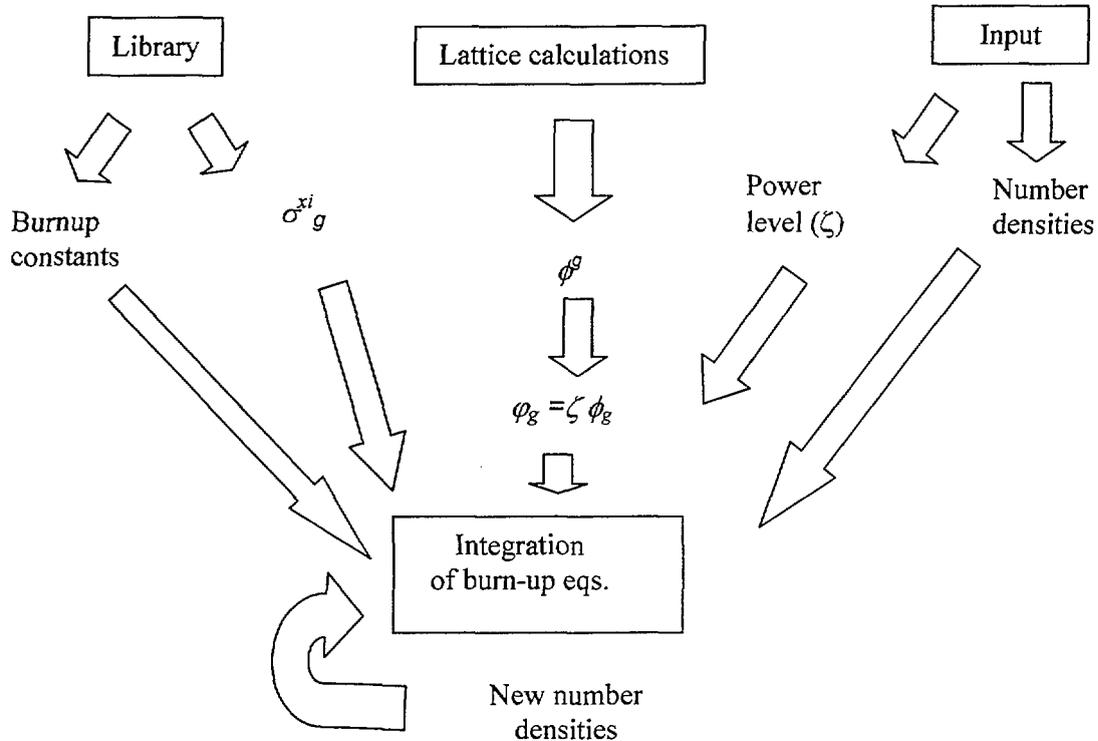
Figure 10: General flow of depletion calculations.
