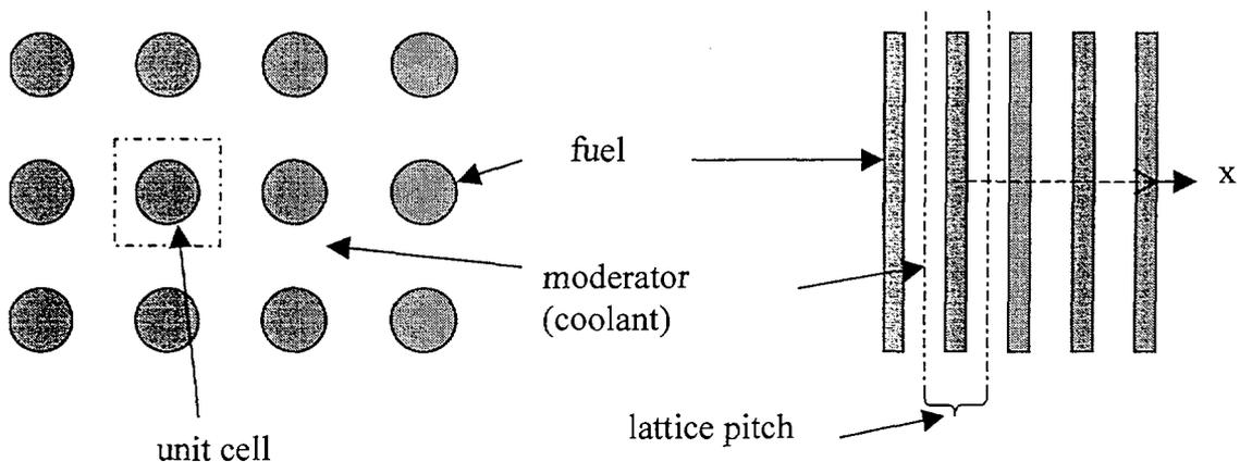
Figure 4: Fragment of a horizontal intersection of a square and plane lattice with a unit cell.
