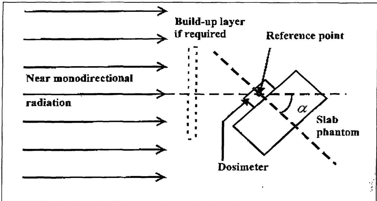
FIG. 2. Arrangement for the calibration of personal dosimeters at angle  $\alpha$ .
